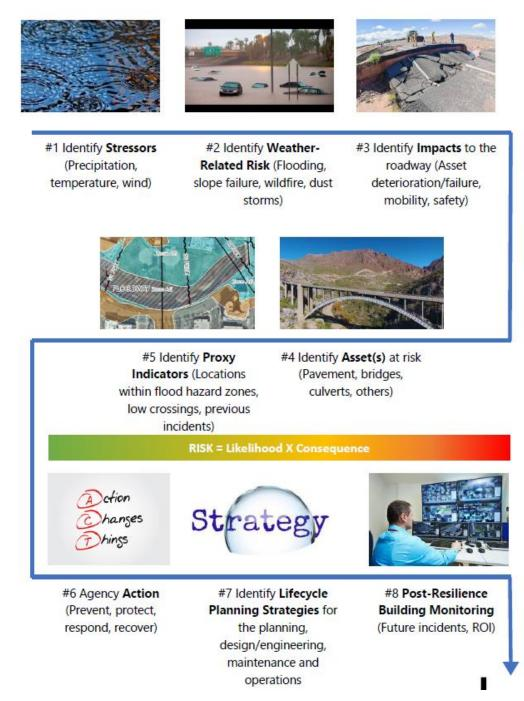
Figure 52. Lifecycle Planning Template Process to Link Extreme Weather Climate Adaptation, Asset Management, and Infrastructure Resilience<sup>5</sup>
