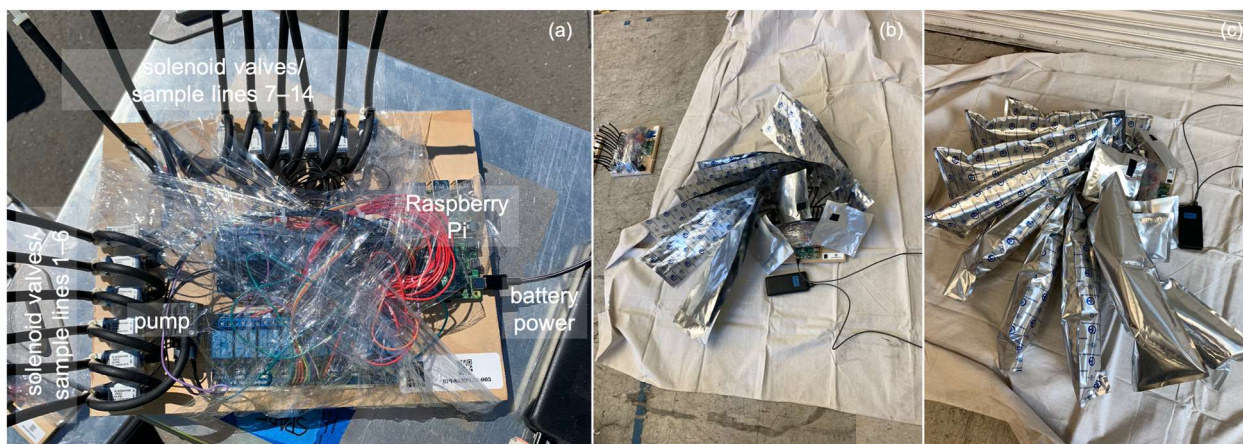
Figure 8. Custom-built samplers used in the South Experimental Area, which semi-continuously filled a series of 0.5 and 10 L multi-layer foil bags to capture 10-min integrated samples during the background, release, transition, and decay period of each experiment. As indicated in (a), the battery-powered system used a programmed Raspberry Pi to control the order, duration, and sampling frequency of up to 14 integrated samples. As also shown in Figure 7, the sampler and attached bags were covered with a drop cloth on the ground (b), as the filled bags (c) could not fit inside the standard aluminum sampler boxes.
