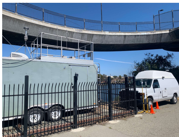
Figure 10. The instrumented research van collocated with the BAAQMD monitoring station to compare the upwind and downwind measurements.
