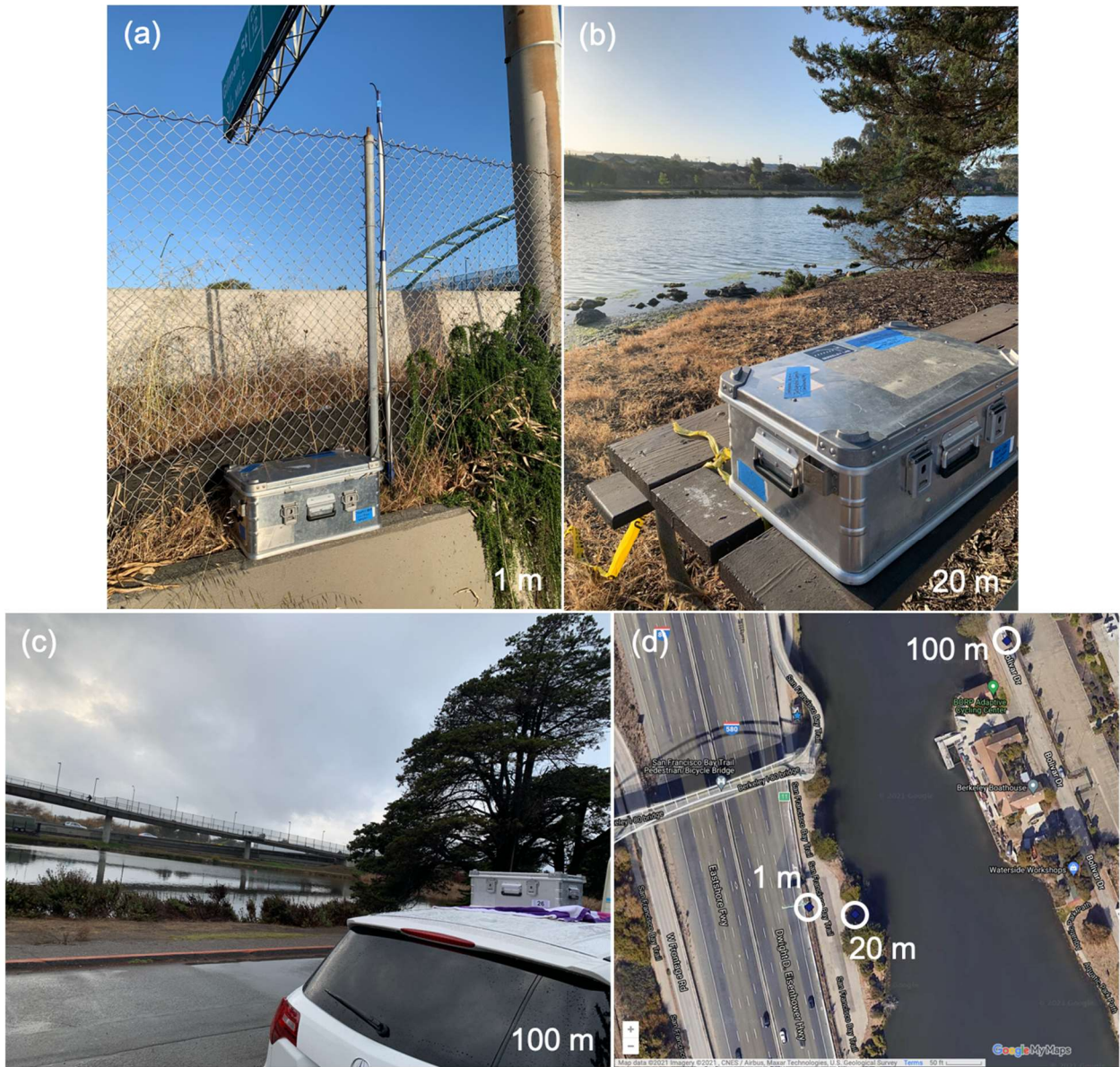
Figure 5. In the North Experimental Area, samplers were placed at downwind target distances of (a) 1, (b) 20, and (c) 100 m. All inlet heights were >1 m above ground and were placed away from potential obstructions that would bias sampled air flow.
