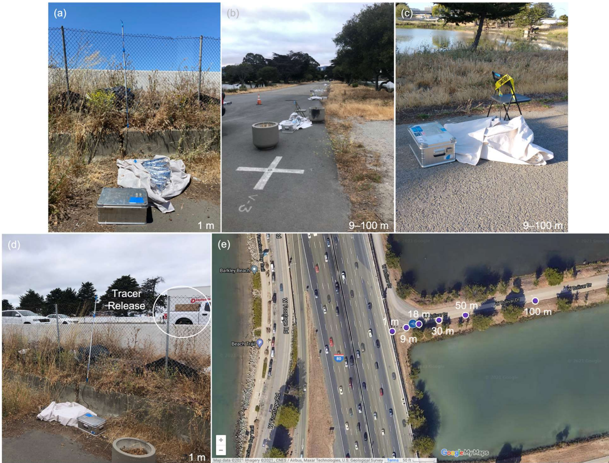
Figure 7. In the South Experimental Area, samplers were placed at downwind target distances of 1, 9, 18, 30, 50, and 100 m. The inlet height at the 1 m distance (a) was extended to a height about 3 m above the sampling area ground level, while the inlets of all other samplers were elevated to about 0.7 m on the backs of folding chairs (b, c). Note the passing mobile tracer release platform in (d) relative to the elevated inlet for the nearest highway sampler also shown in (a).
