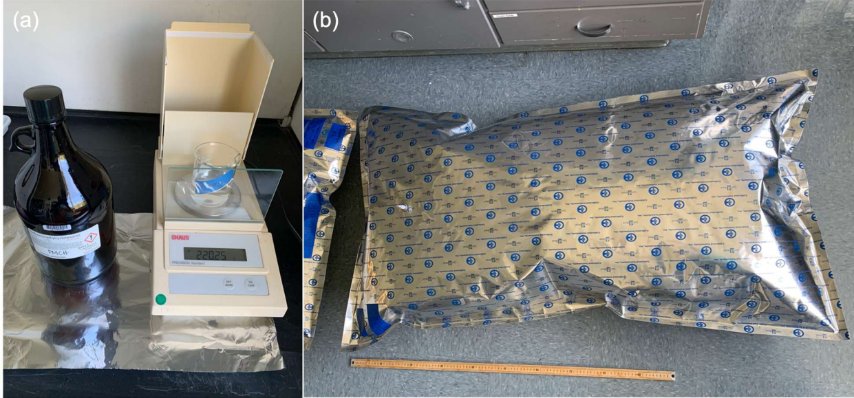
Figure 3. Laboratory preparation of tracer source bags, including (a) weighing the tracer material to be injected into the bag and (b) the final bag size after being filled with ultrahigh purity N_2 and the liquid tracer had evaporated.
