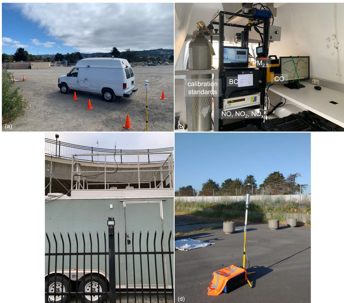
Figure 9. Concentrations of key air pollutants and wind speed/direction were measured upwind and downwind of the tracer release experiments. (a) At the upwind site, measurements were made with a 2D sonic weather sensor and an instrumented research van with a sample inlet on the roof oriented towards the San Francisco Bay. (b) Concentrations of NO, NO 2 , NO x , CO, PM 2.5 , and BC were measured with analyzers housed in the van, and instrument response was verified daily with gas calibration standards and particle filters. (c) Downwind concentrations of the same pollutant species were measured at the BAAQMD's Berkeley Aquatic Park monitoring station in the North Experimental Area, including a PM 2.5 analyzer that the Berkeley team temporarily installed on the station's perimeter fence. (d) Downwind measurements of wind speed were made with a 3D sonic anemometer in the South Experimental Area.
