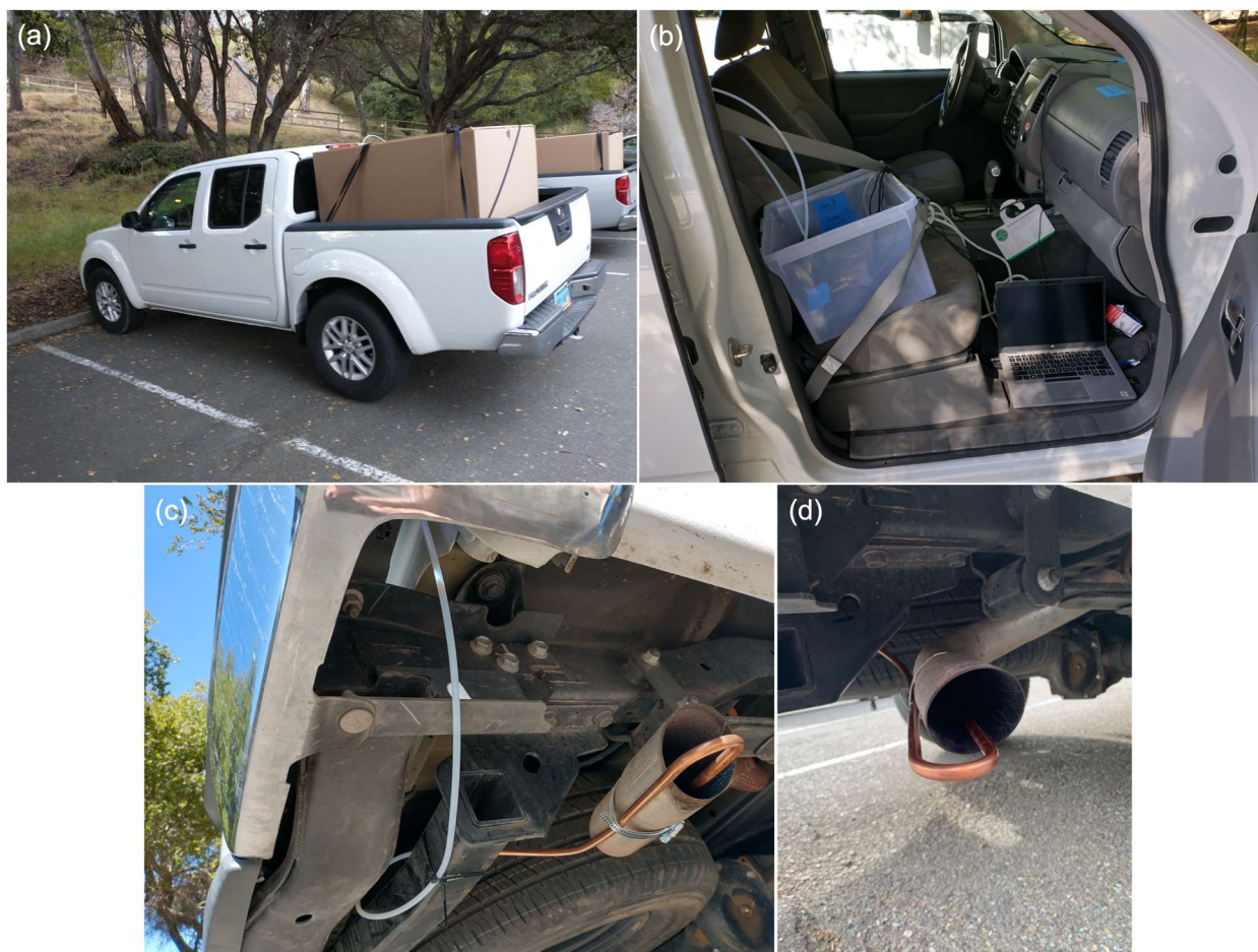
Figure 4. Tracer release system installed on one of the vehicles that served as a mobile platform during the experiment. (a) The source bag was secured within a large cardboard box in the bed of the pickup truck. (b) The PFT + N 2 mixture was pumped out of the source bag through 1/4" Teflon tubing, through the automated system that was housed in the bin on the passenger seat, including the pump, flow meter, and Raspberry Pi controller. The GPS was secured on the vehicle's dash and the laptop that logged pump flow rate and GPS data was placed on the floor. (c) The PFT gas flowed through a second stretch of 1/4" Teflon tubing along the side of the truck bed and down to the tailpipe, where 3/8" copper tubing was installed. (d) This copper tubing was bent into a U-shape into the truck's tailpipe so that tracer gas was co-emitted with the truck's exhaust at temperature.
