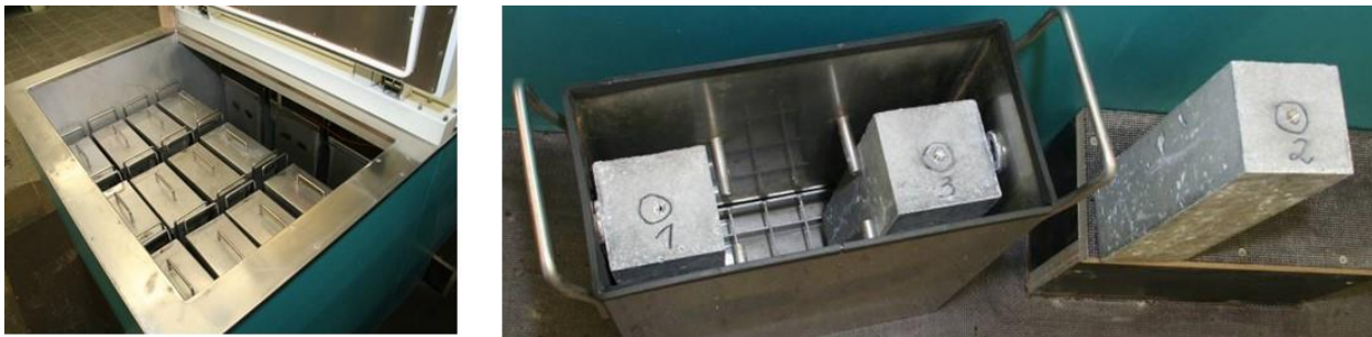
Figure 19. Reactor generating 60 °C (140 °F) and 100% humidity (left). Sealable containers suitable for the AAR-11 for storing concrete prisms (right). (RILEM, 2018c).
