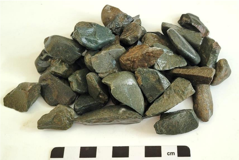
Figure 1 : Siltstone (Aggregate Sudbury).
