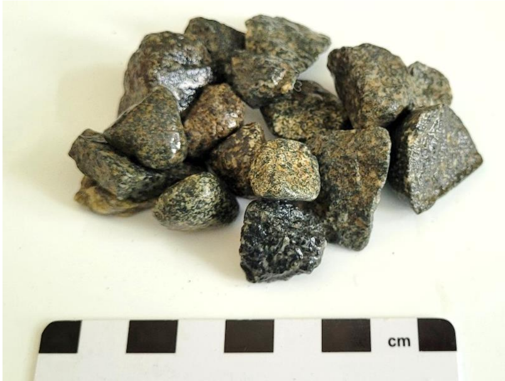
Figure 3: Granite (Aggregate Sudbury).
