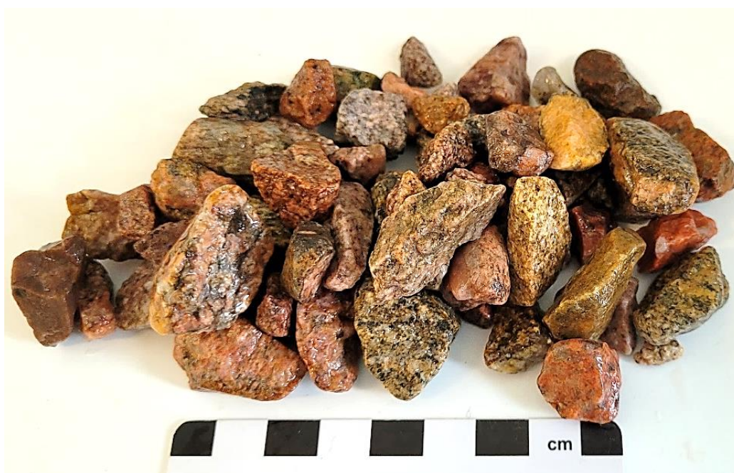
Figure 2: Gneiss granitique (Aggregate UT-06).
