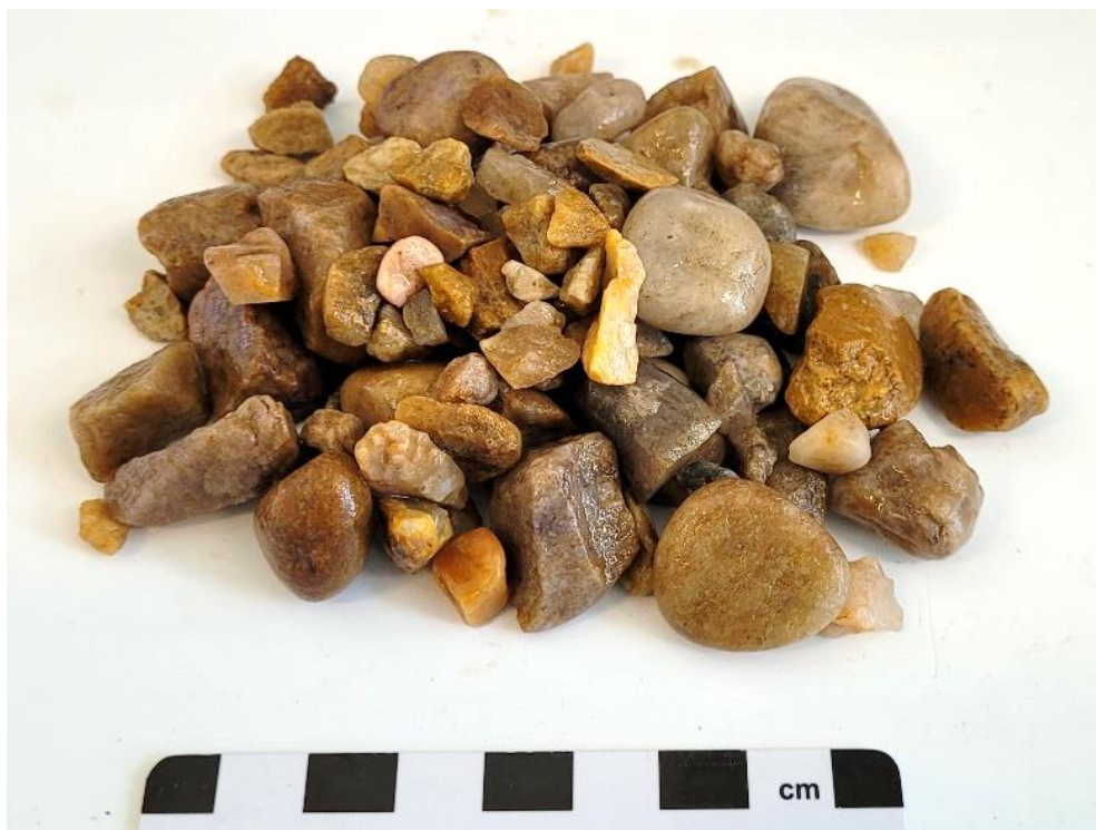
Figure 3: Quartzite (Aggregate Placitas)
