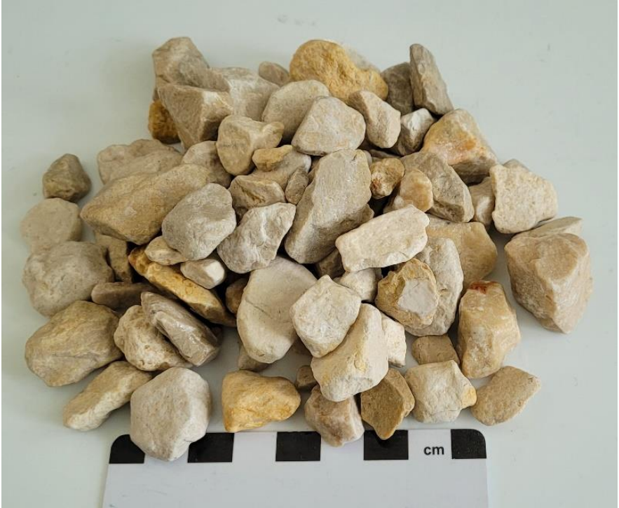
Figure 1 : Light-grey to beige limestone (Aggregate NR1).
