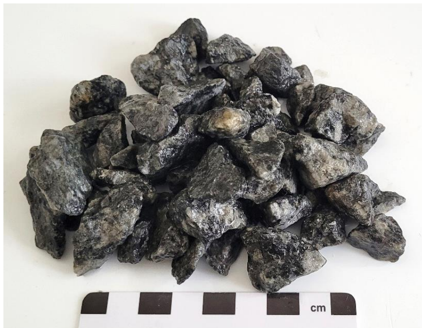
Figure 1 : Metagranite (Aggregate CA4).
