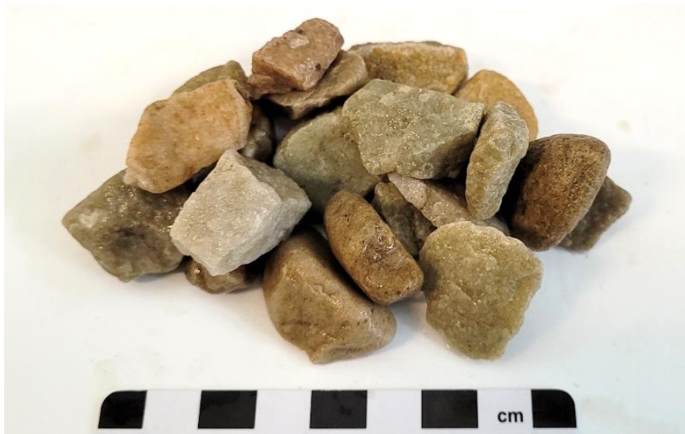
Figure 4: Graywacke (Aggregate Sudbury).
