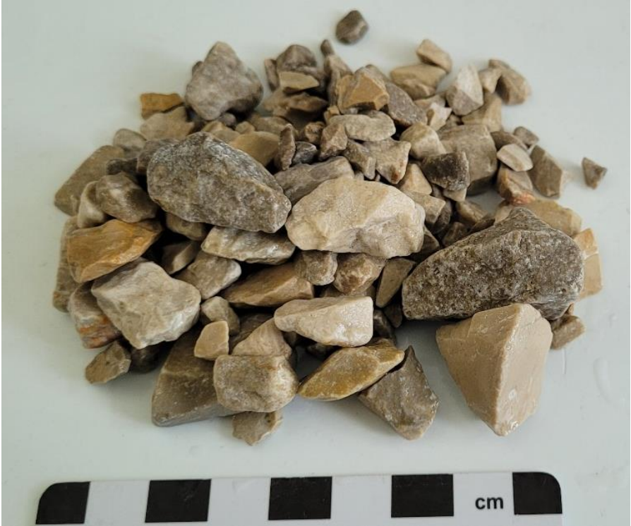
Figure 2: Medium-gray limestone (Aggregate NR1).
