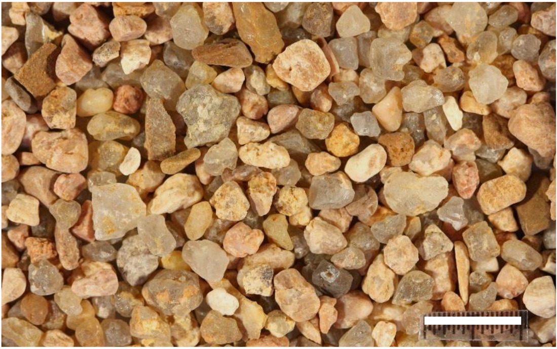
Figure 1 : Photographs of the fine Aggregate RAT1. A & B: fraction 4 – 8 mesh (2.36 – 4.75mm). The scale on the photographs is 10 mm.
