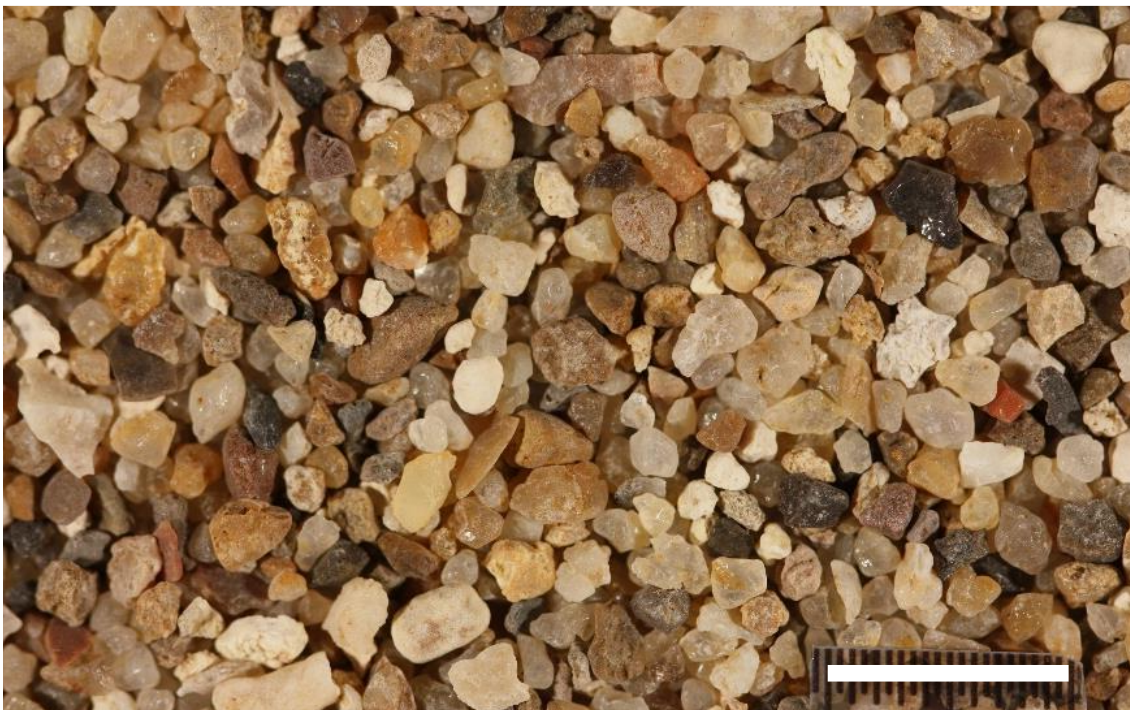
Figure 2 : Photographs of the fine Aggregate RAT2. A & B: fraction 8 – 16 mesh (1.18 – 2.36 mm). The scale on the photographs is 10 mm.
