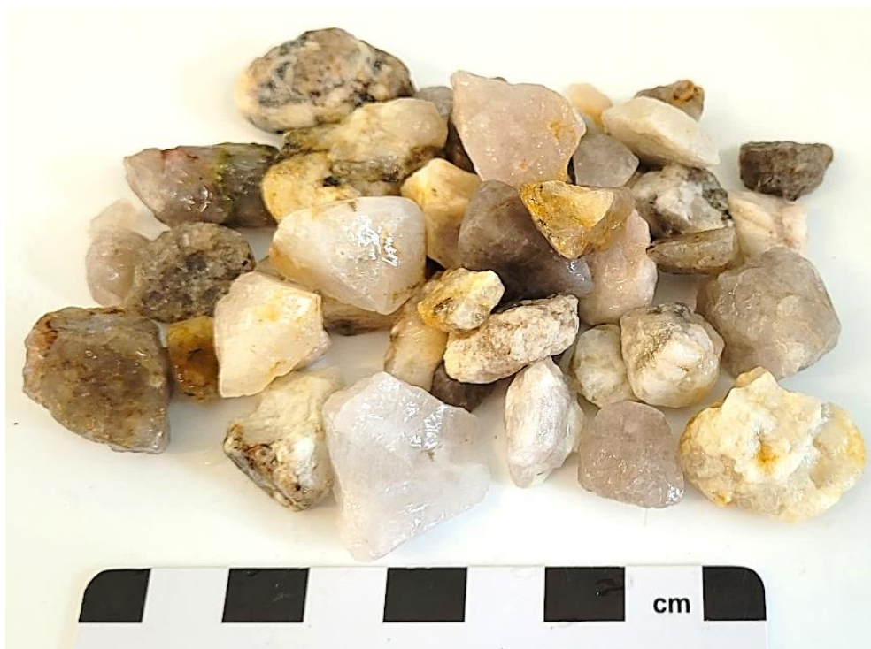
Figure 3: Quartz veins (Aggregate CA2).
