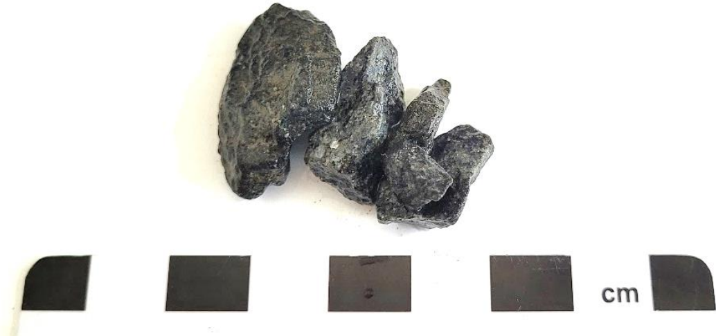
Figure 2: Granitic gneiss (Aggregate CA4).
