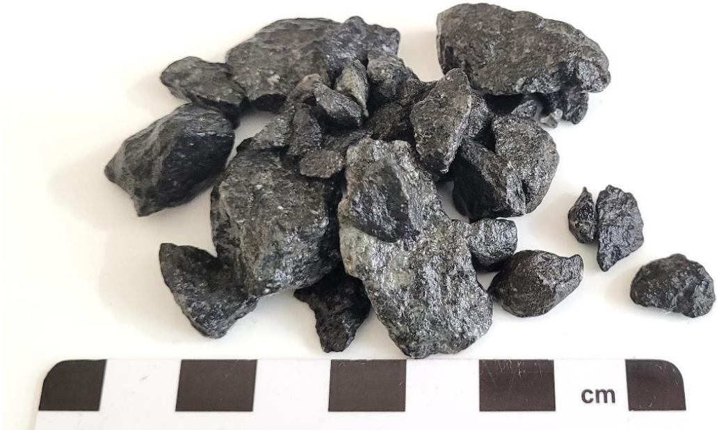
Figure 2: Fine-grained metagranite (Aggregate CA1).
