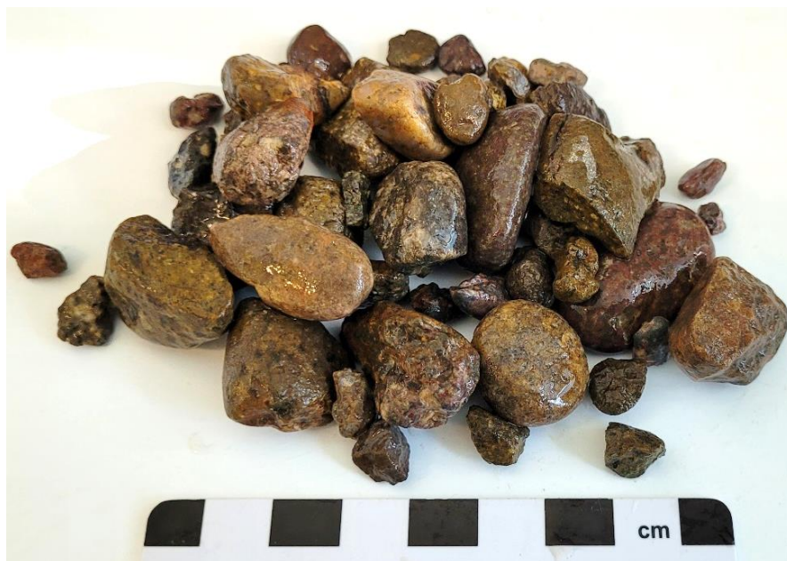
Figure 1 : Andesite - basalt (Aggregate Placitas).
