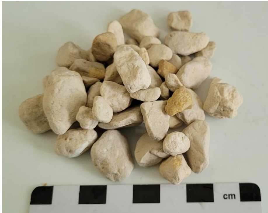
Figure 4: Altered limestone (Aggregate NR1).
