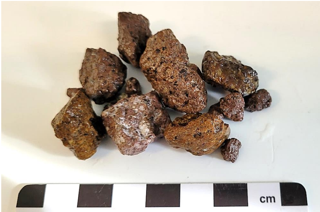
Figure 5: Rhyolite (Aggregate CA2).
