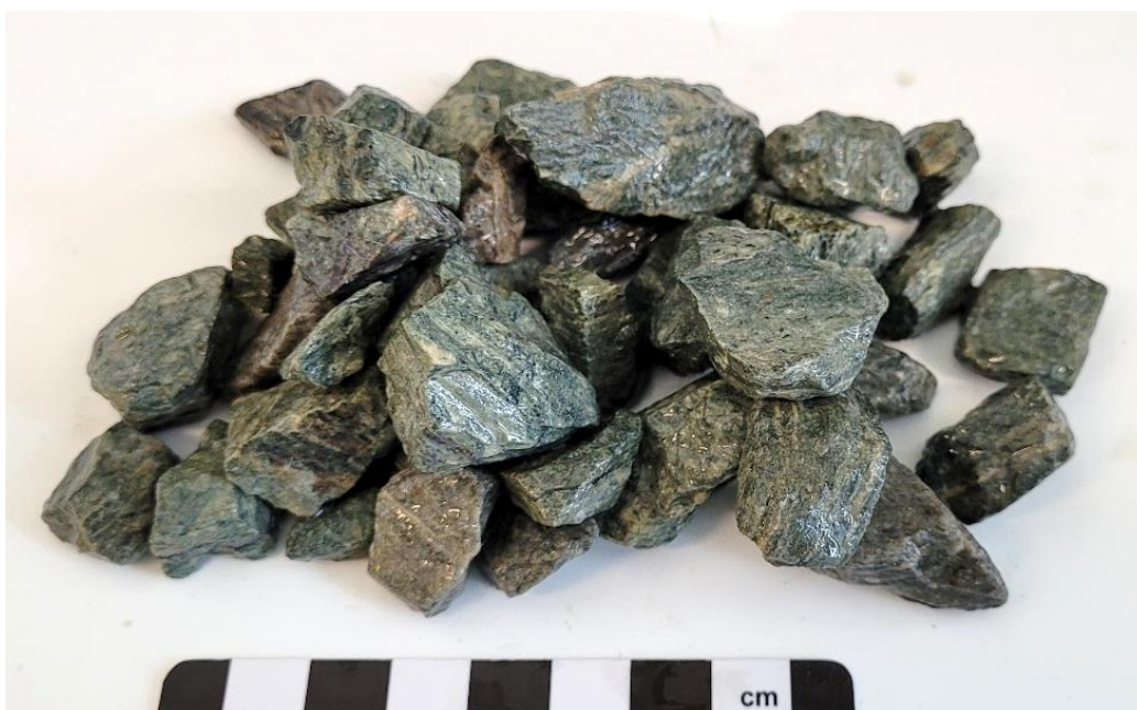
Figure 2: Fine-grained green schist facies (Aggregate CA3).
