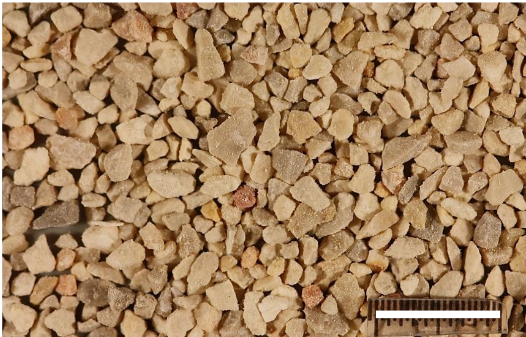
Figure 2 : Photographs of the fine Aggregate NR2. A & B: fraction 8 – 16 mesh (1.18 – 2.36 mm). The scale on the photographs is 10 mm.
