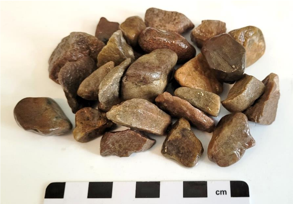
Figure 2: Sandstone (Aggregate Sudbury).
