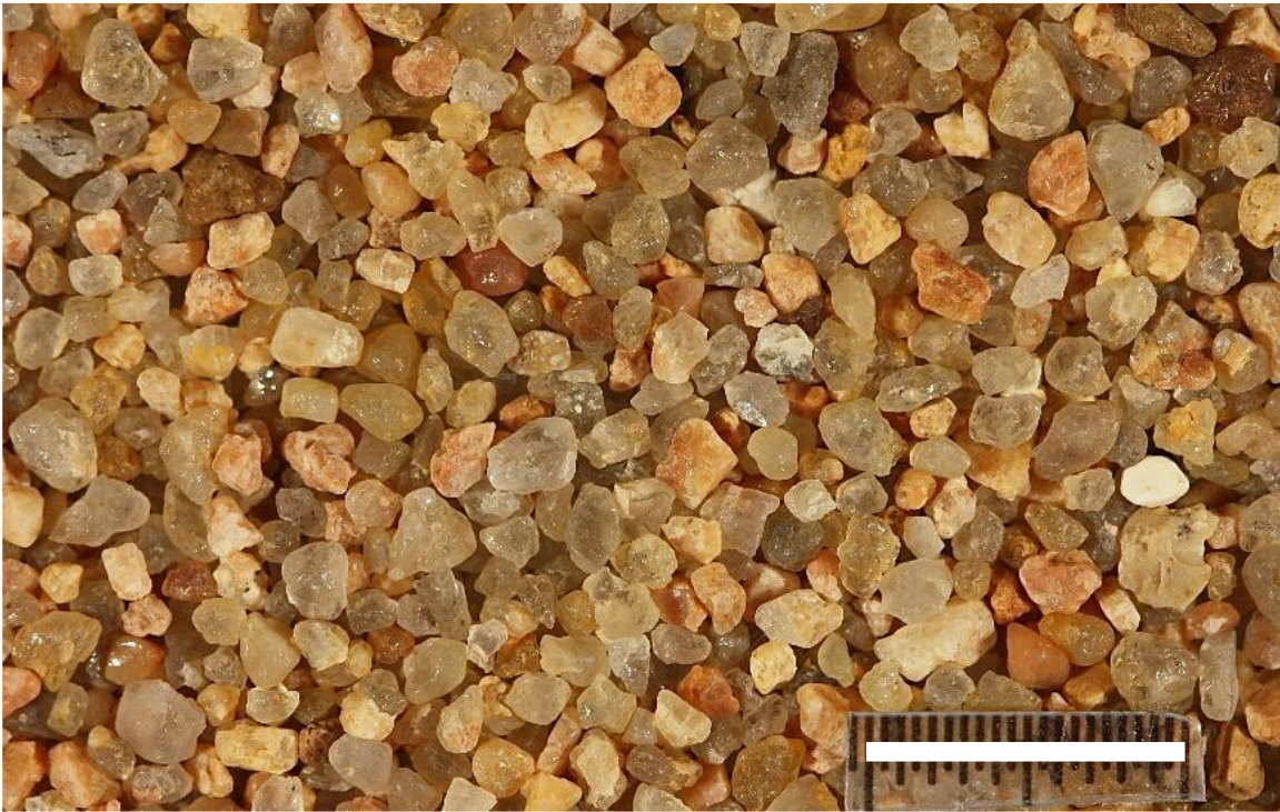
Figure 2 : Photographs of the fine Aggregate RAT1. A & B: fraction 8 – 16 mesh (1.18 – 2.36 mm). The scale on the photographs is 10 mm.
