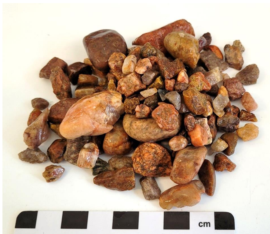
Figure 2: Quartz and feldspar veins – “granitic/gneissic” material (Aggregate Placitas).
