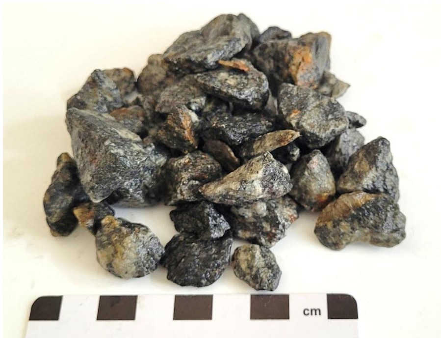
Figure 3: Rusted metagranite (Aggregate CA1)
