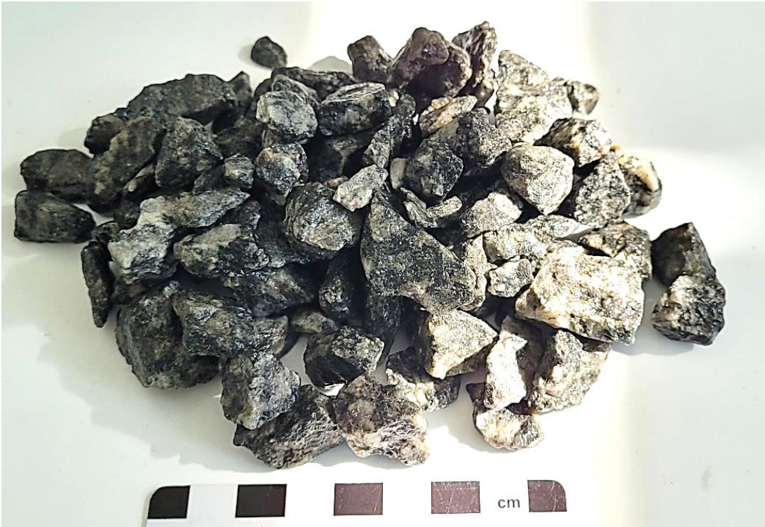
Figure 1 : Metagranite (Aggregate CA1).
