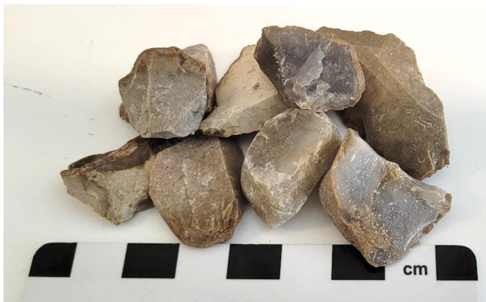
Figure 4: Chert (Aggregate CA2).
