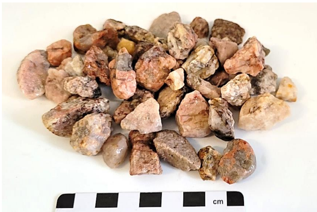
Figure 1 : Granite (Aggregate CA2).
