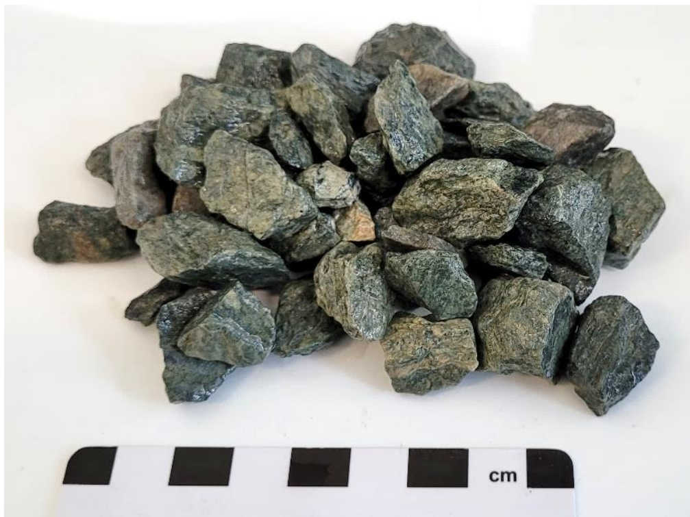
Figure 1 : Green schist facies (Aggregate CA3).
