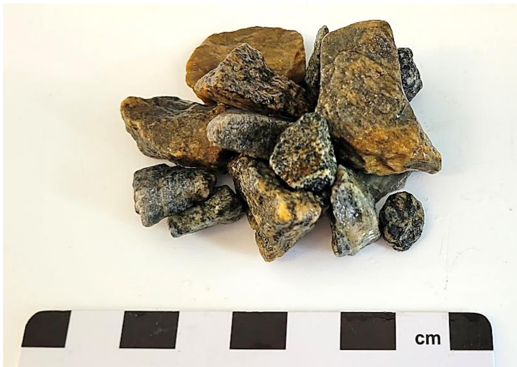
Figure 6: Sandstone (Aggregate CA2).
