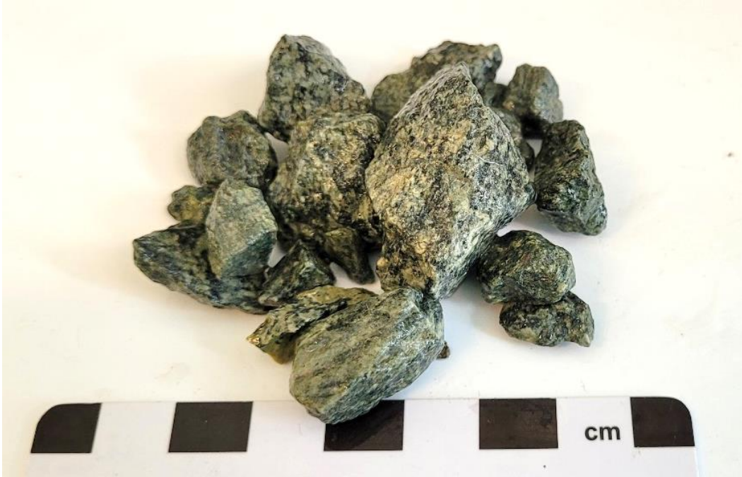
Figure 3: Altered green schist facies (Aggregate CA3).
