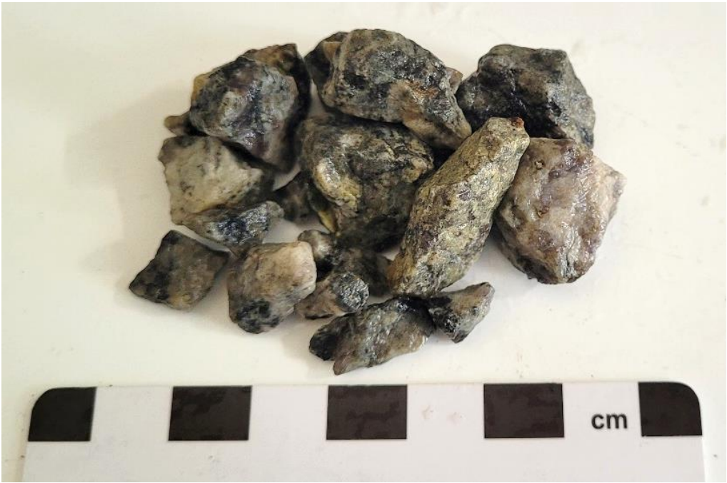
Figure 3: Epidote and quartz vein (Aggregate CA4).
