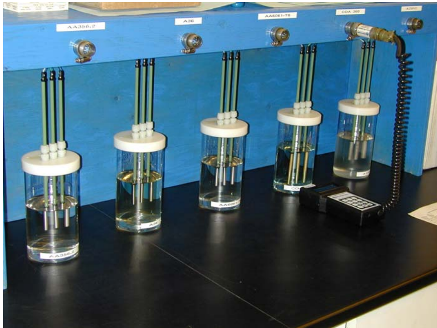
Figure A-1 – General View of LPR Test Arrangement with Meter Affixed to Brass (CDA 360) Samples
