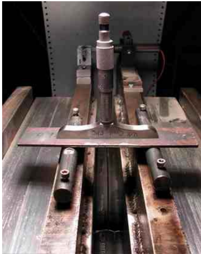
Figure C-10 Depth Gauge Shown Measuring Bulge
