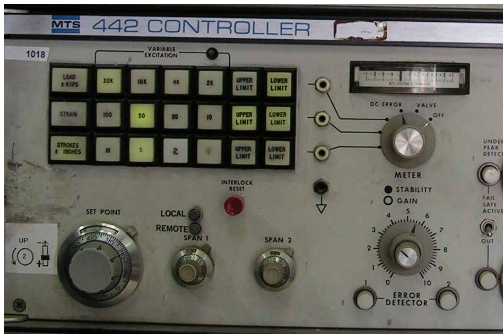
Figure 9 MTS Controls with Set Point Dial in Lower Left and Meter in Upper Right
