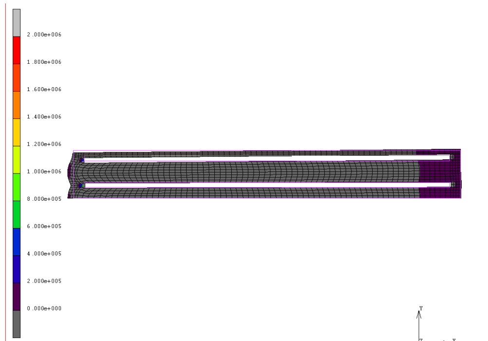
Figure E-41 Tensile hydrostatic stress in (Pa) for \sigma = 0.445 GS and \theta_y = 0.0060 rad/layer
