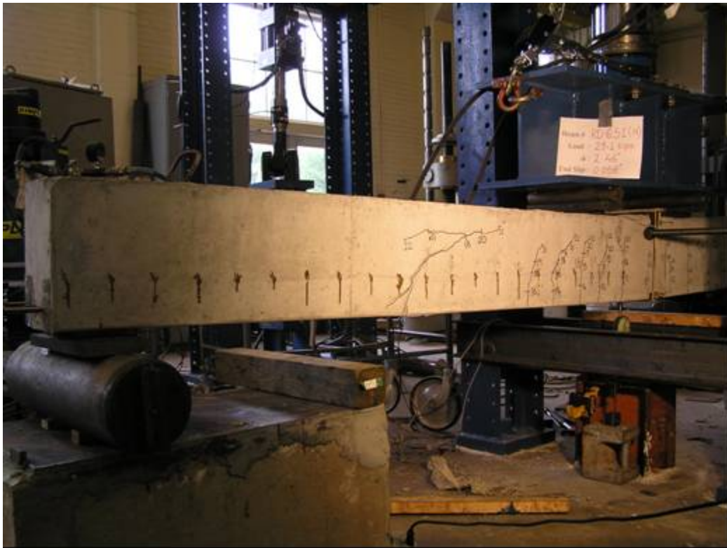
Cracking pattern for Beam RD-6-5-1 being loaded at North end.
