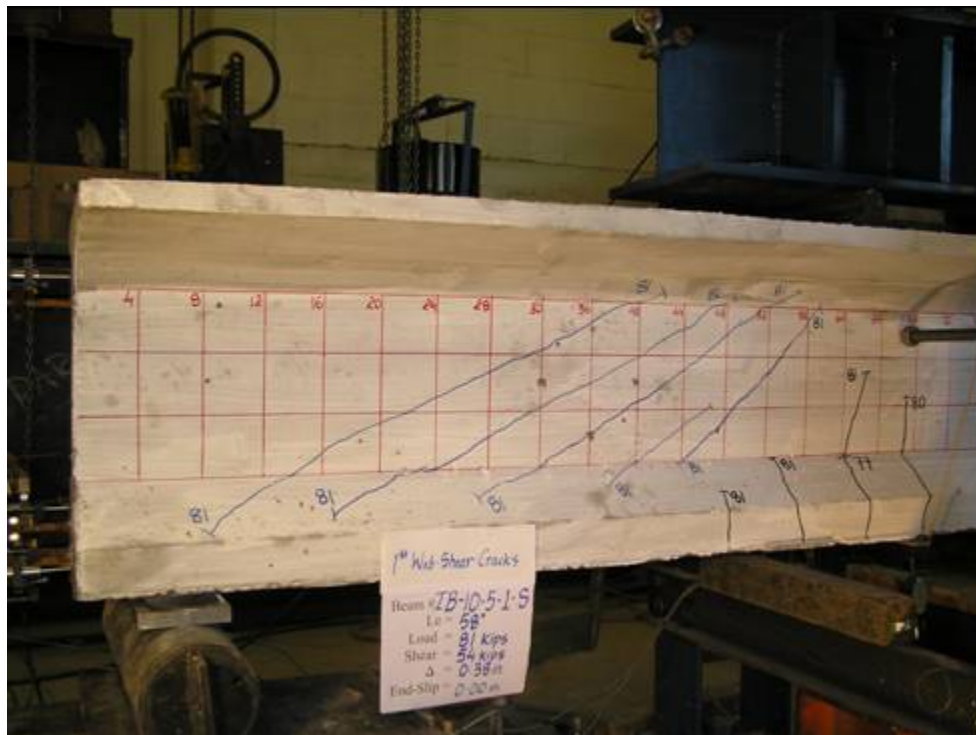
Photo of the South end of the beam IB-10-5-1 showing the first web shear cracking
