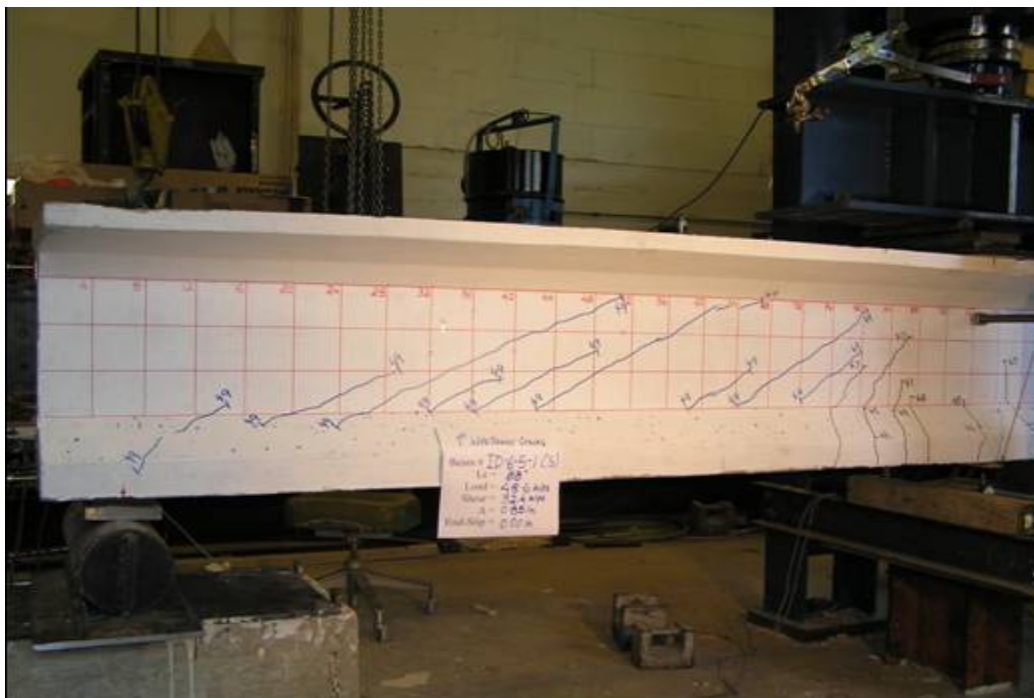
Photo of the South end of the beam ID-6-5-1 showing the first web shear cracking
