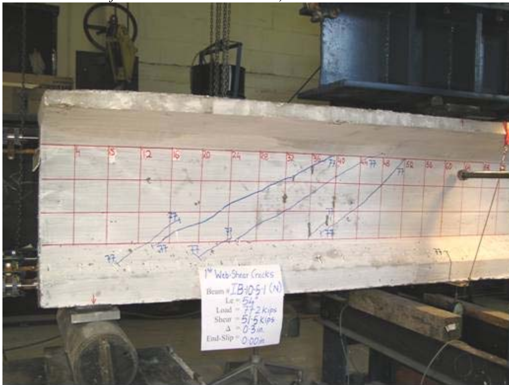
Photo of the North end of the beam IB-10-5-1 showing the first web shear cracking incidentally the point of first flexural cracking as well)
