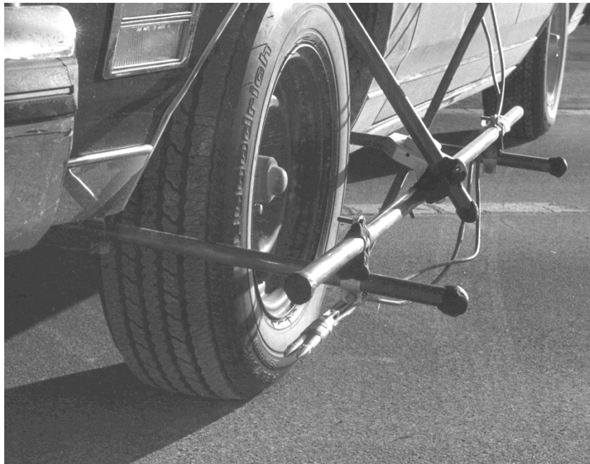
Figure 13: Early application of sound Intensity to mapping source regions of a passenger car tire (57)
