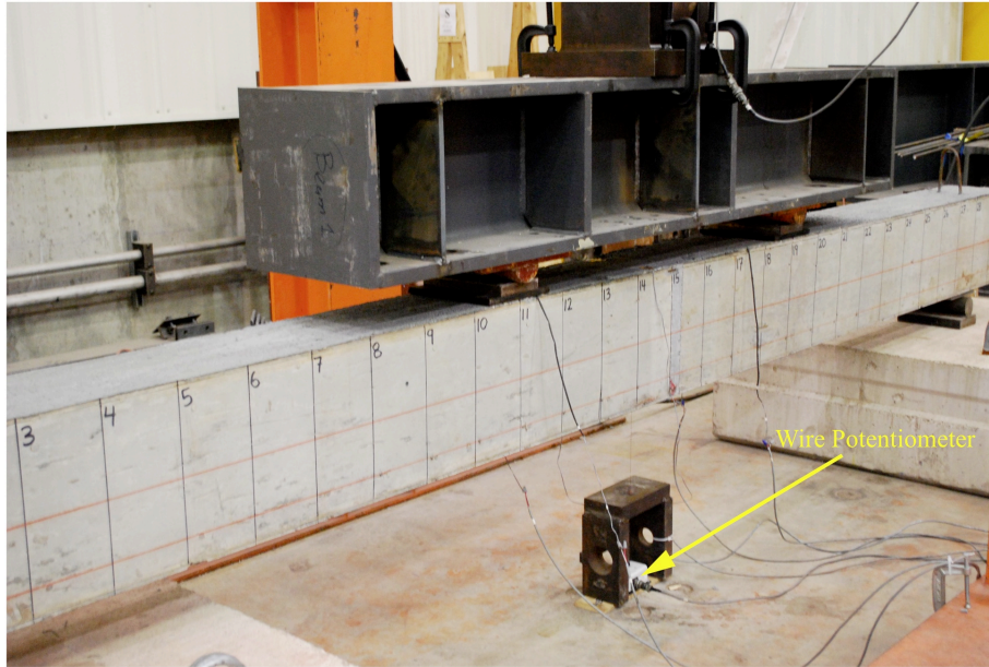
Figure H4 Instrumentation for Measuring the Midspan Deflection
