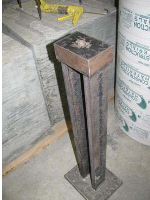
Figure 3. Steel frame used for loading
