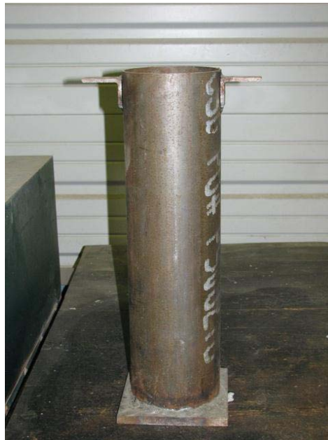
Figure 2. NASP specimen before filling (welded plate, angles are visible)
