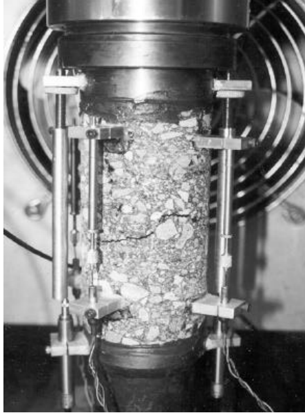
FIGURE 95 Specimen test setup (Daniel and Kim, 2001).
