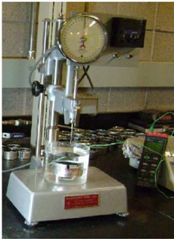
FIGURE 45 Penetration test apparatus and specimen preparation.
