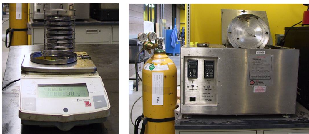
FIGURE 41 PAV equipment and specimen preparation.
