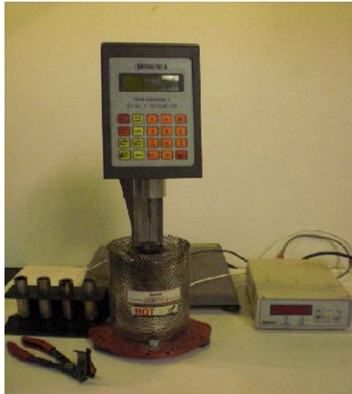
FIGURE 47 Brookfield test apparatus and specimen preparation.
