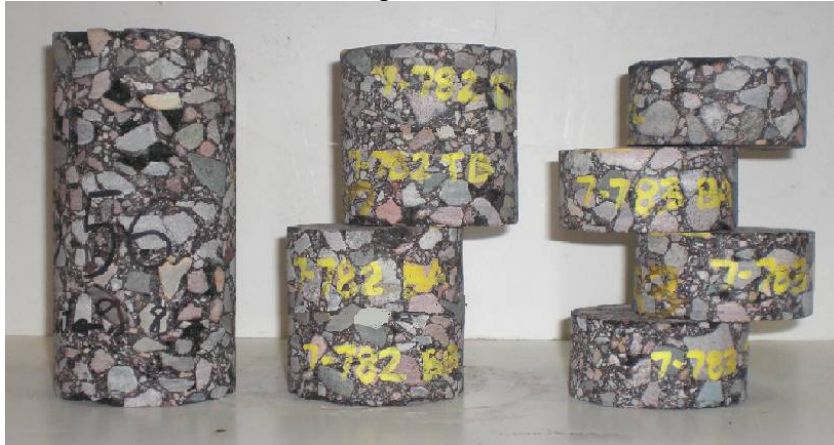
FIGURE 105 Steps of specimen cutting for different air voids calculations.
