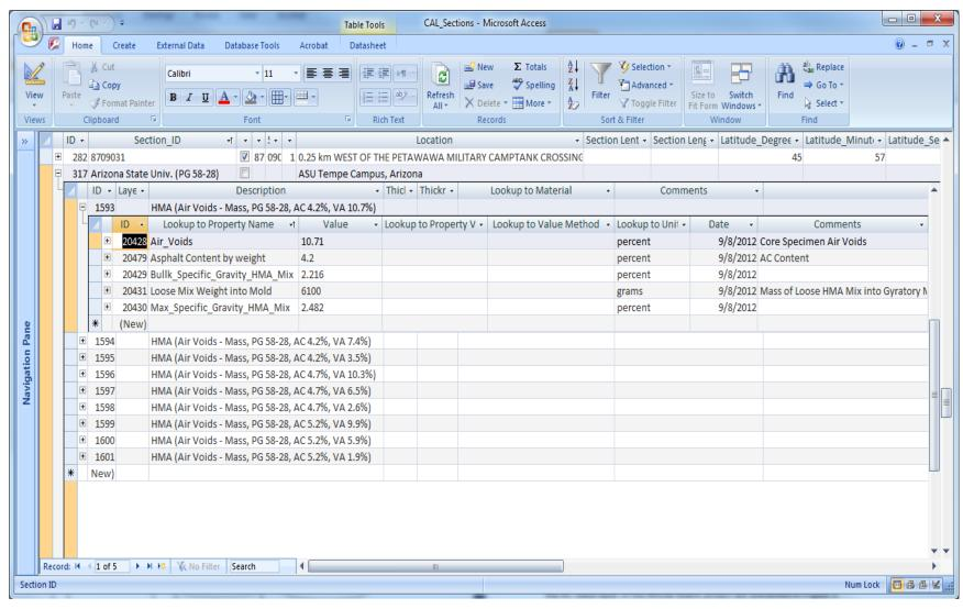
Figure 8 Screenshot of the Database: Air Voids-Mass Data Input
