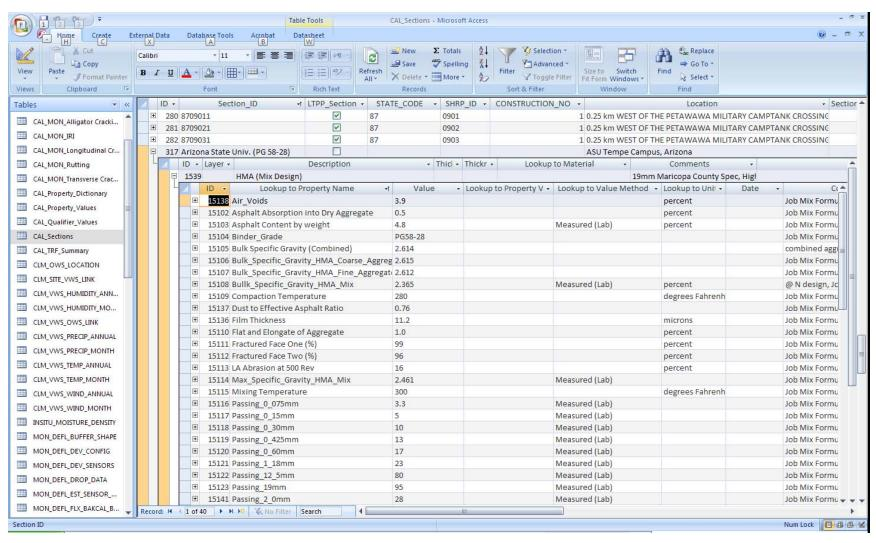
Figure 3 Screenshot of the Database: Mix Design Data Input
