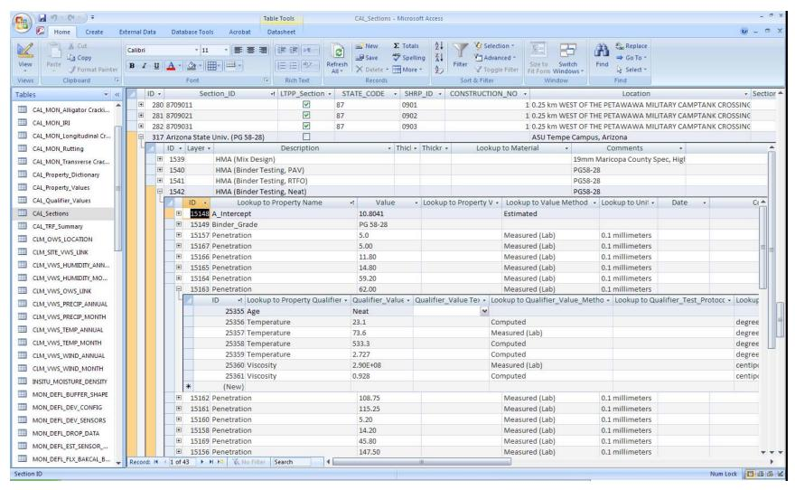
Figure 4 Screenshot of the Database: Binder Test Results Input
