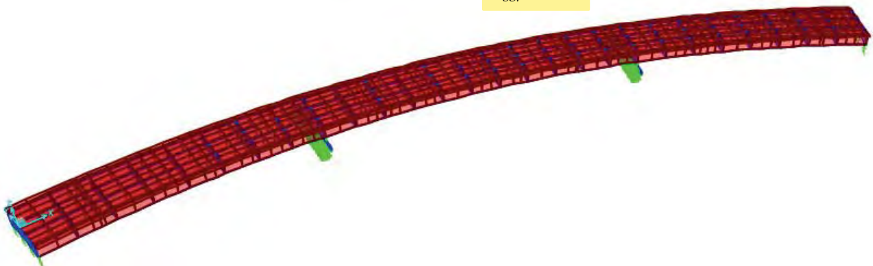
Figure 2: Screenshot of the 3D analysis model
