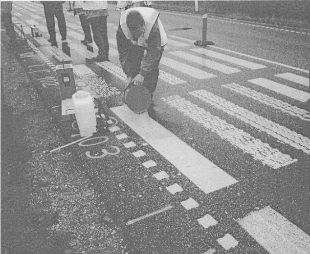
FIGURE 23 CEN procedure for wetting the marking for wet simulation testing. (Source: Flint Trading Company, Inc.)
