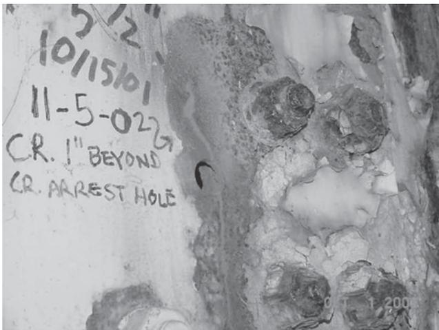
FIGURE A8 Magnetic particle testing—Indication.
