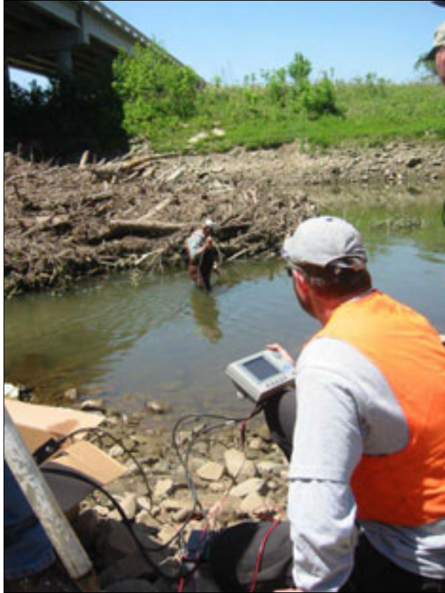
Figure 4.6. Using the Twinscope to map the underwater configuration of the debris pile.
