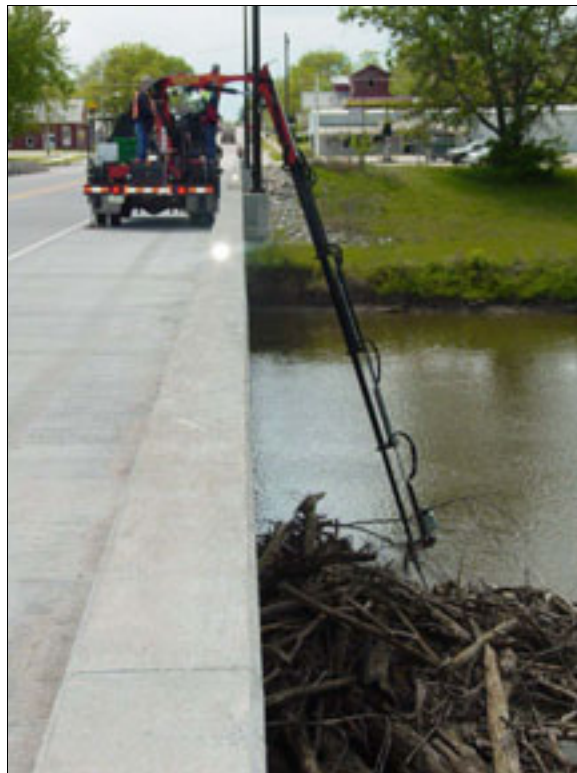
Figure 1.8. Articulating arm truck with crane extended to take measurements.
