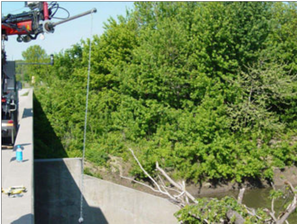
Figure 3.10. Using the chain and steel ball extension to obtain elevations of the debris pile.
