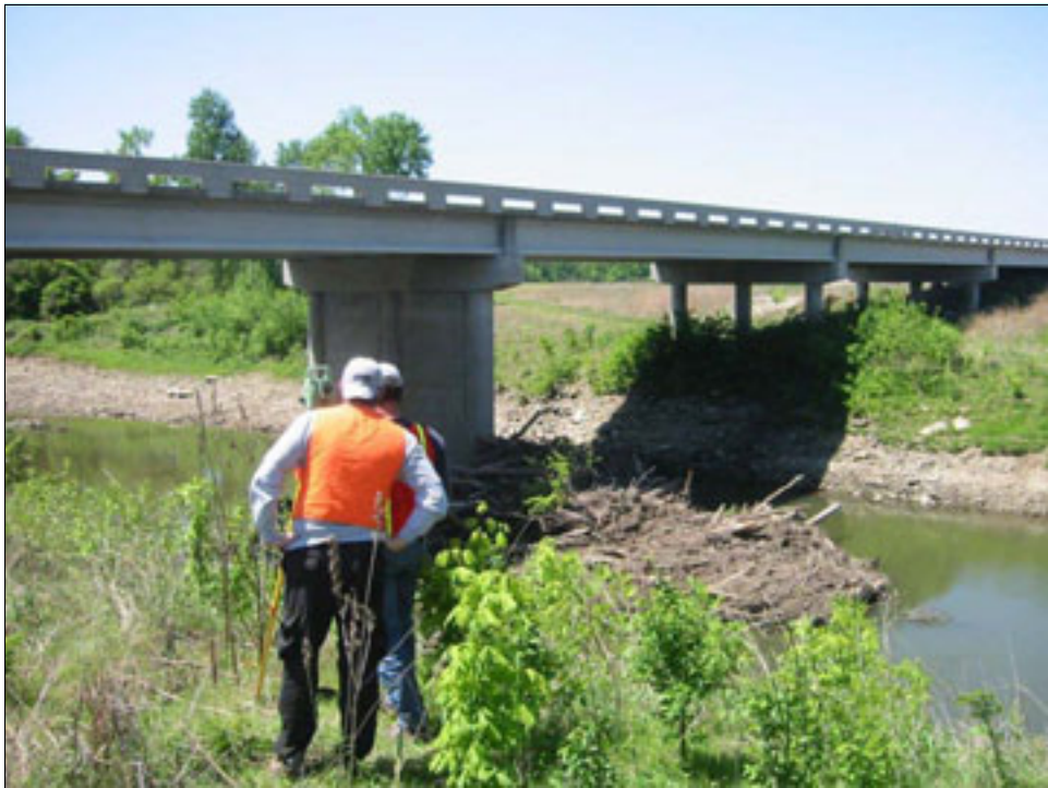
Figure 4.5. Surveying the debris pile with the total station.
