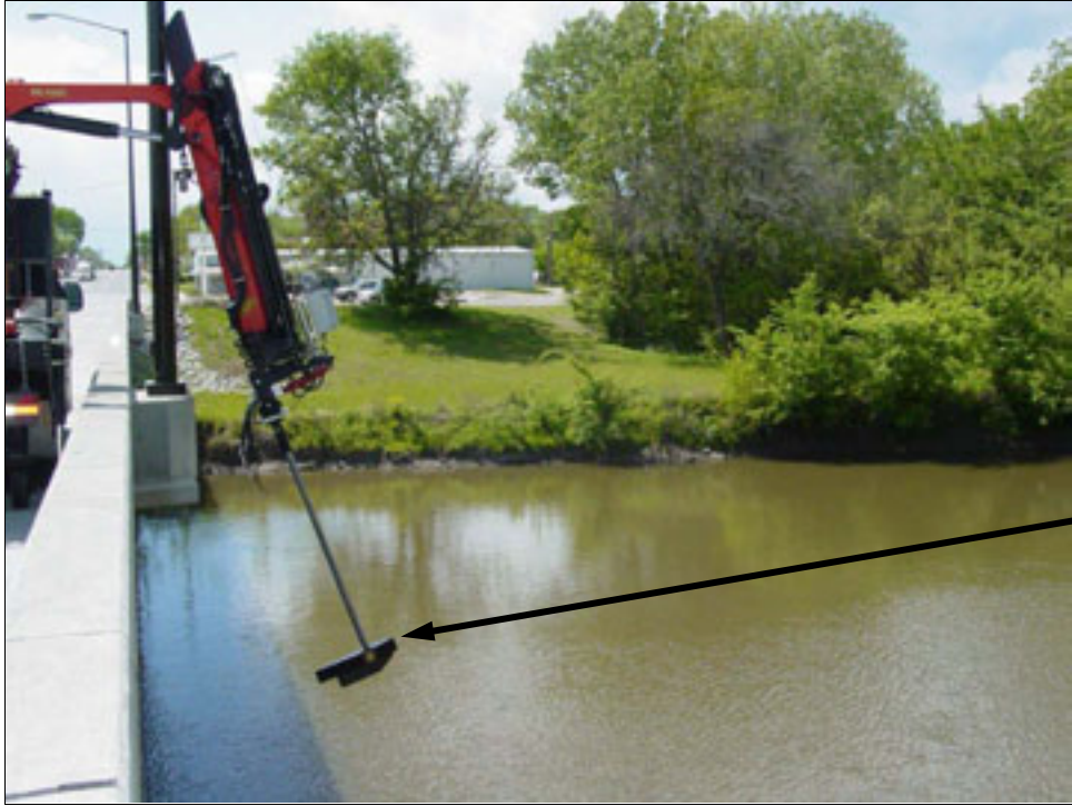
Figure 1.11. Streamline probe to position wireless sonar.
