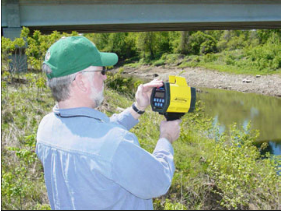
Figure 4.8. Using the laser range finder.
