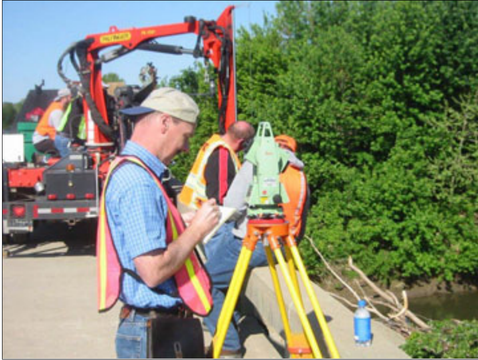
Figure 3.9. Using the Leica total station with data logger.
