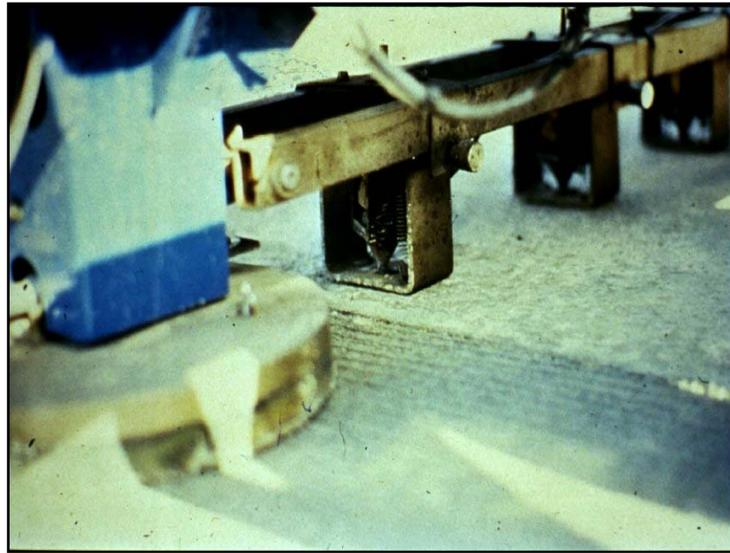
Figure 11. Falling weight deflectometer load plate and deflection sensors.
