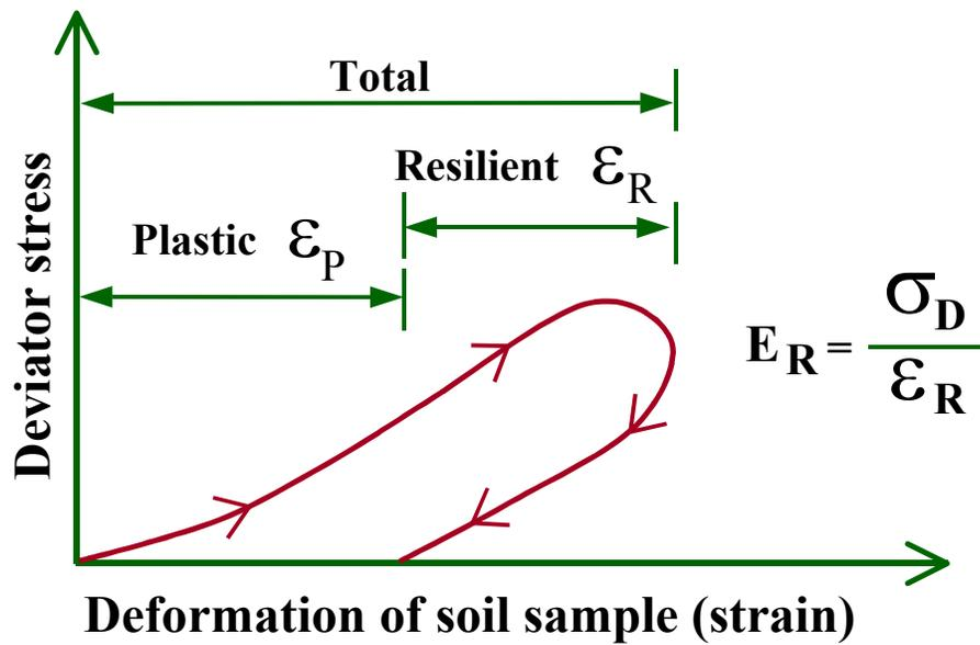
Figure 13. Resilient modulus concept.<sup>18</sup>
