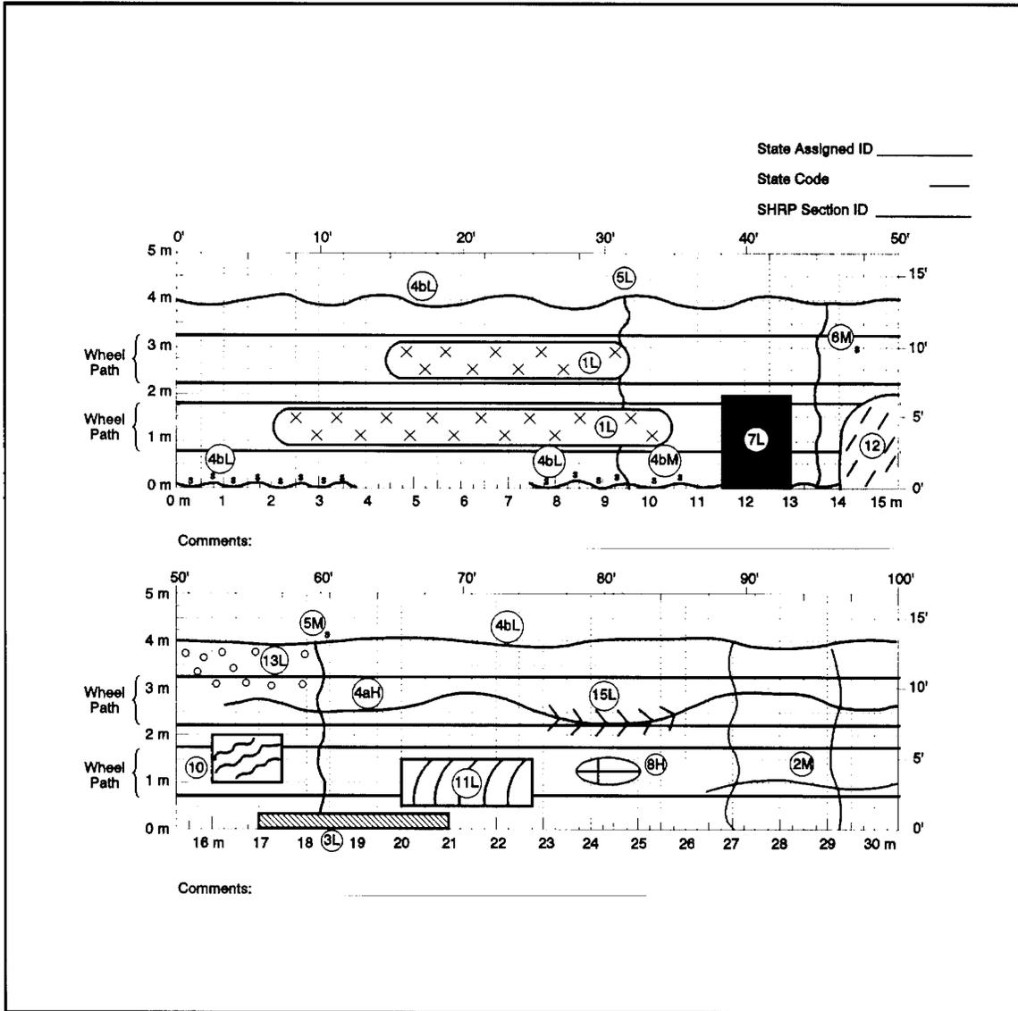
Figure 2. Example distress survey map for asphalt pavement.<sup>11</sup>
