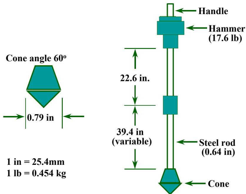
Figure 14. Diagram of Dynamic Cone Penetrometer (DCP).<sup>18</sup>
