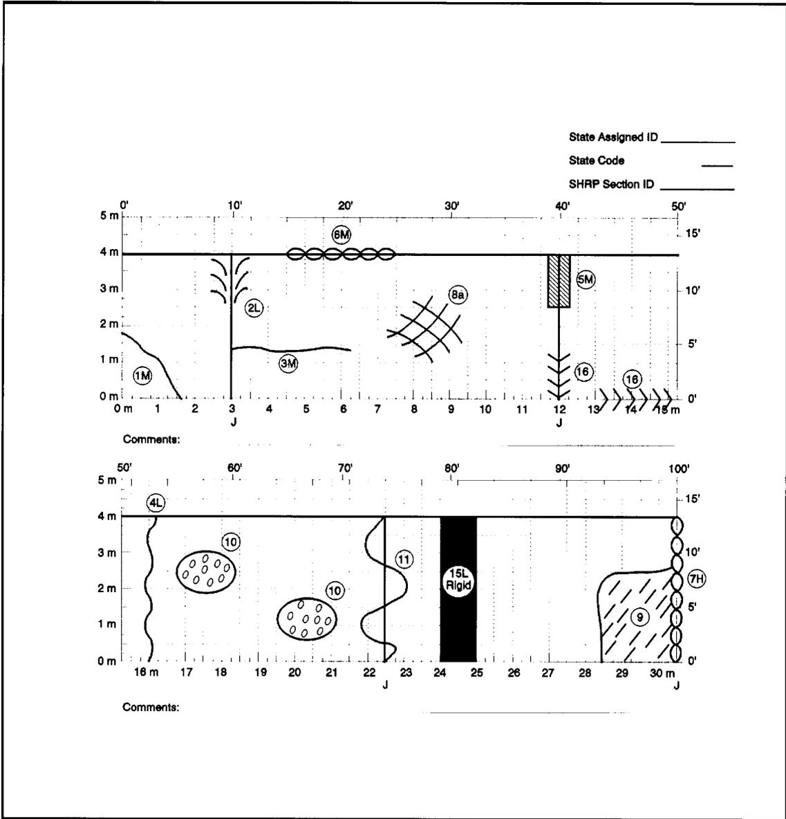
Figure 4. Example distress survey map for jointed concrete pavement.<sup>11</sup>
