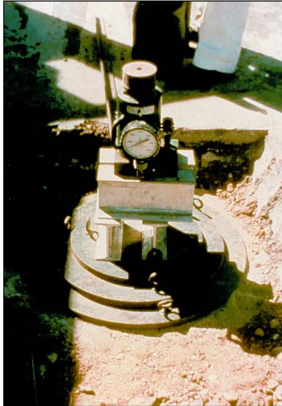
Figure 16. Photo of plate load testing apparatus.
