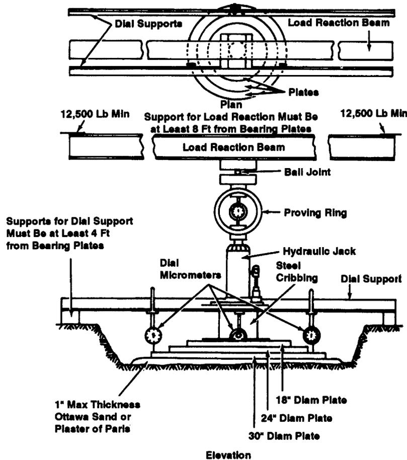
Figure 15. Diagram of plate load testing apparatus.<sup>14</sup>
