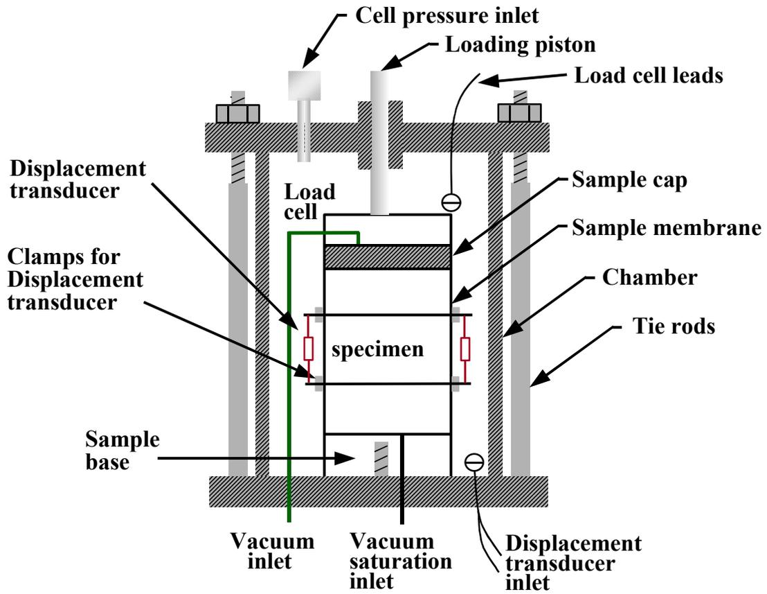
Figure 12. Resilient modulus testing apparatus for soils.<sup>18</sup>
