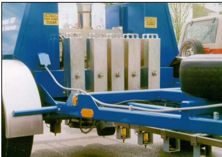
Figure 10. Load package and sensor bar on falling weight deflectometer.
