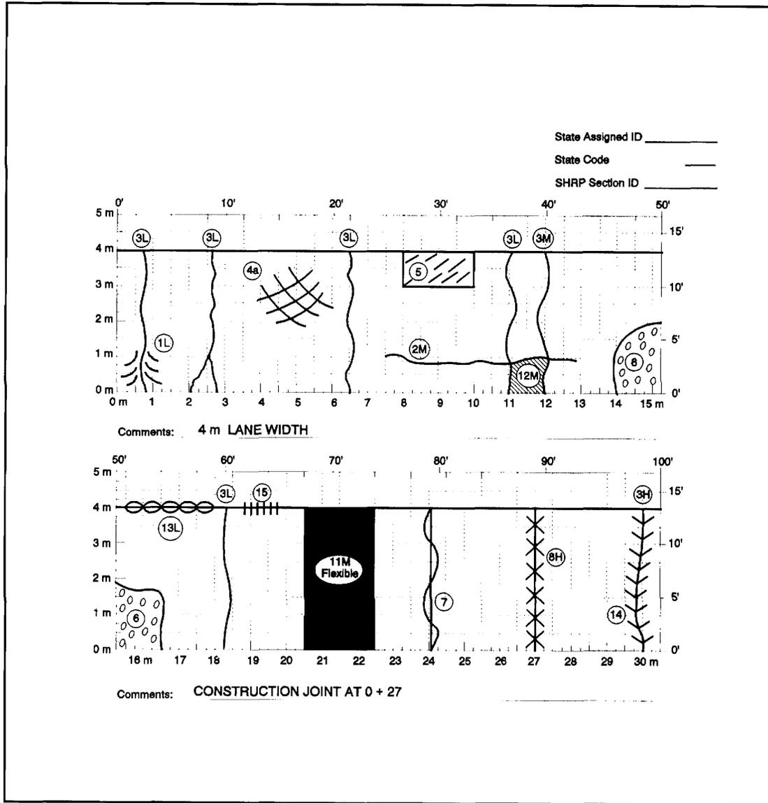
Figure 6. Example distress survey map for continuously reinforced concrete pavement.<sup>11</sup>
