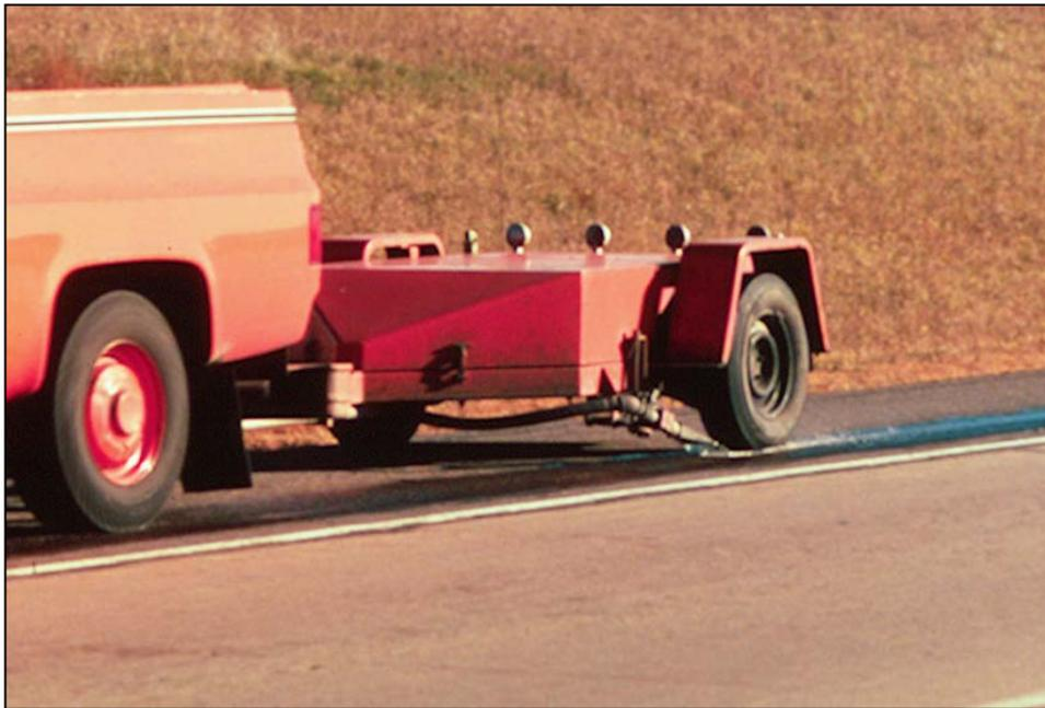
Figure 18. Locked-wheel friction testing.
