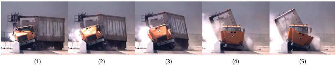
Figure 10: Illustration of collision sequence in tractor-semitrailer impacts with longitudinal barriers (Test TL5CMB-2)[Rosenbaugh07]
