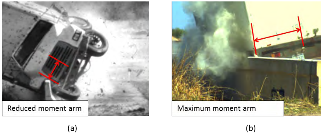
Figure 35. Full-scale crash tests illustrating engagement points of vehicle during redirection for (a) 32-inch tall barriers [Bullard, 2010] and (b) 36-inch tall barriers. [Sheikh , 2011]
