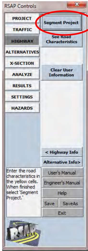
Figure 20. RSAP Controls Dialog Box for Road Segments: Segment Project to estimate encroachments.
