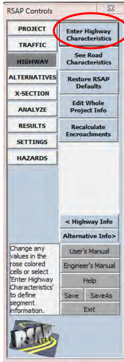
Figure 15. RSAP Controls Dialog Box for Highway Characteristics.
