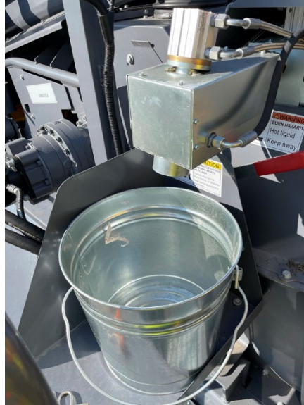
Figure 2. Foaming nozzle and test bucket on a CCPR plant.
