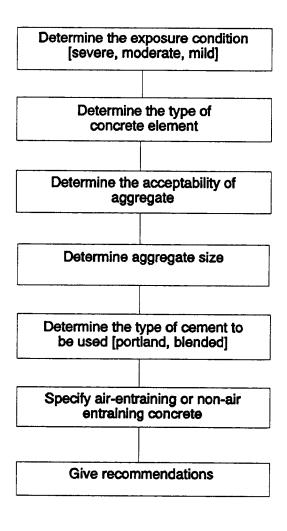
Figure 1. Expert system model for freeze-thaw durability concrete design.
