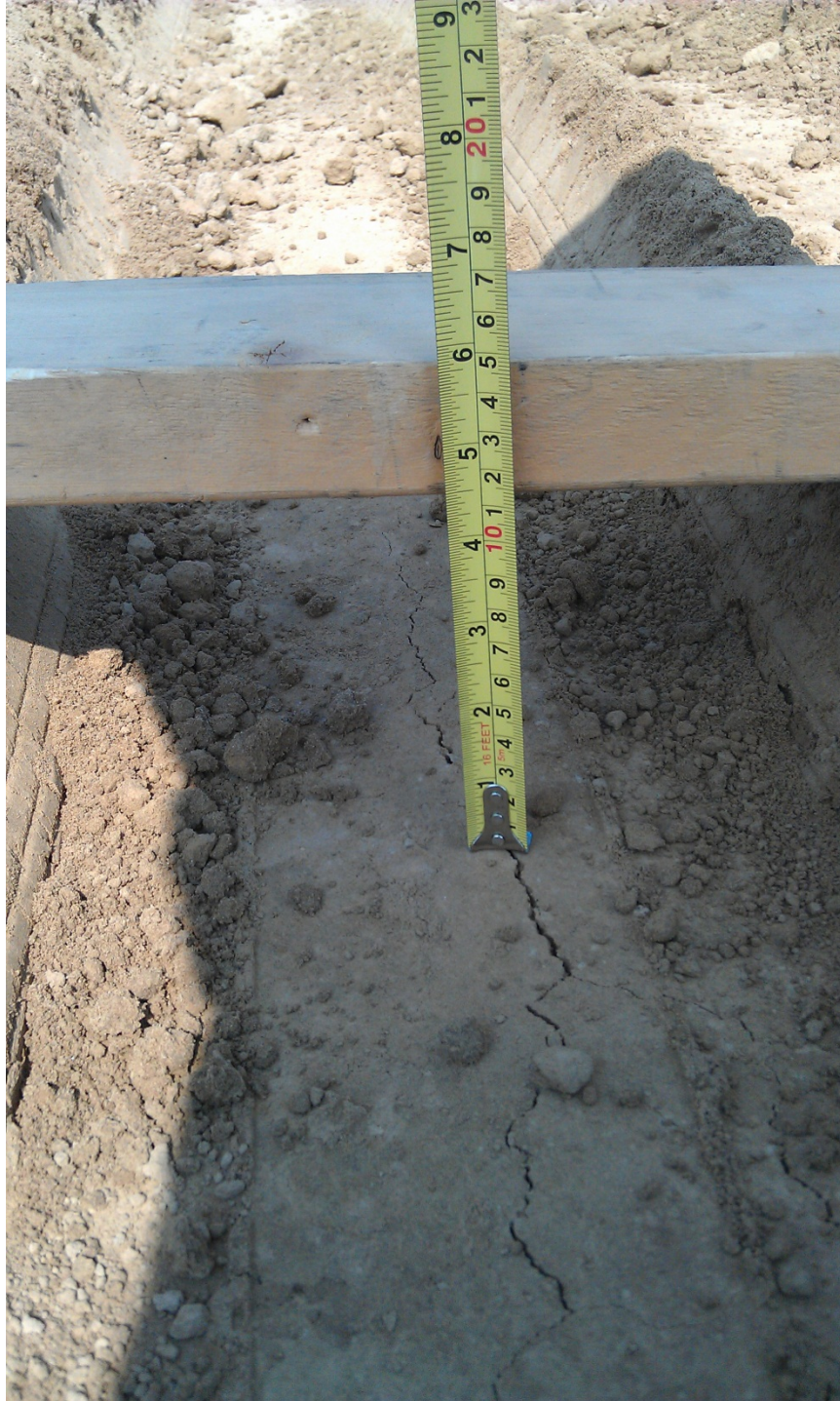
Figure 68: Test area #2—rut measurement
