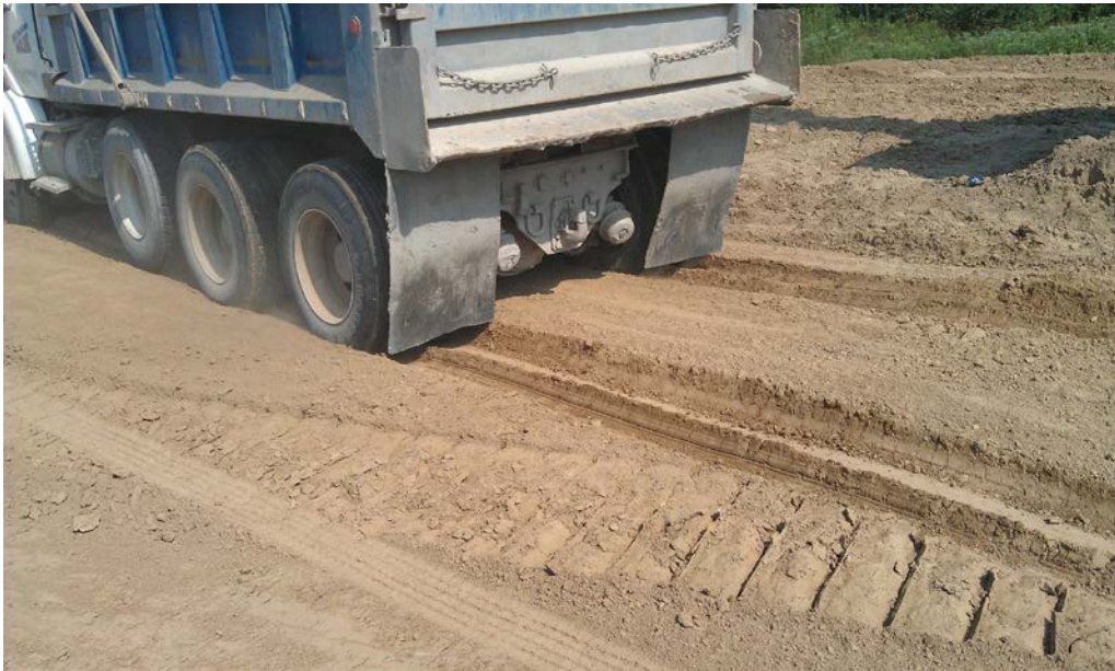
Figure 67: Test area #2—significant rutting
