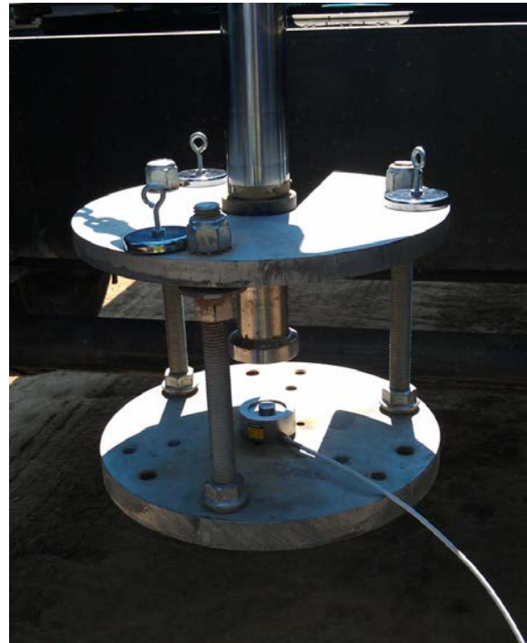
300 mm plate load test setup
