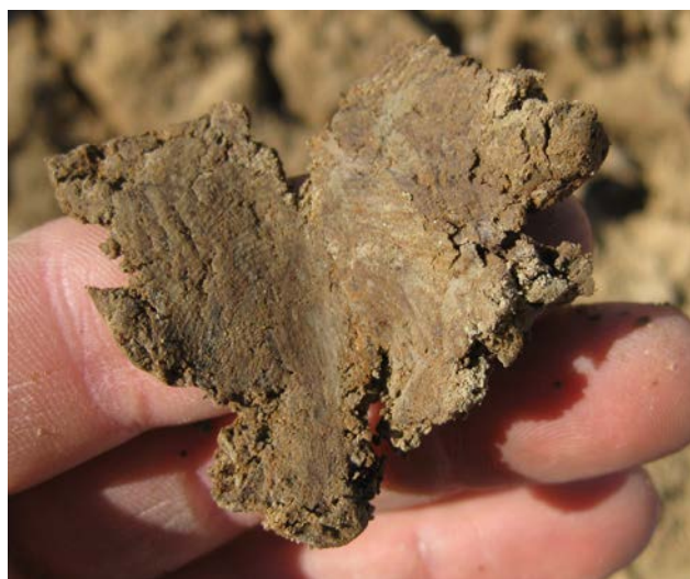
Figure 7: Silty clay embankment fill material
