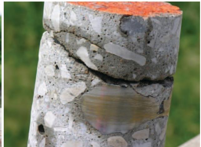
**Figure 2.4.** Delamination observed in extracted cores.
