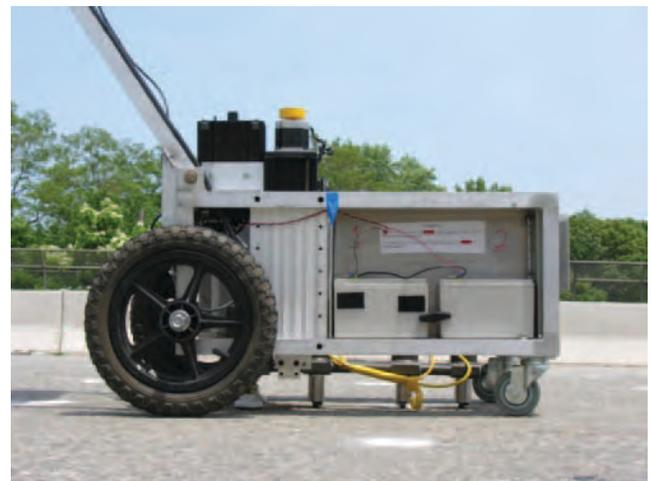
Figure 3.5. USW testing using a portable seismic property analyzer (PSPA).
