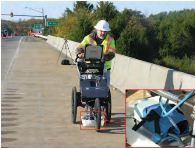
**Figure 3.10. GPR testing.**
