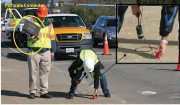
*Figure 2. Illustration of the impulse-response testing with main equipment components: portable computer (left), and instrumented hammer and geophone (right).*
