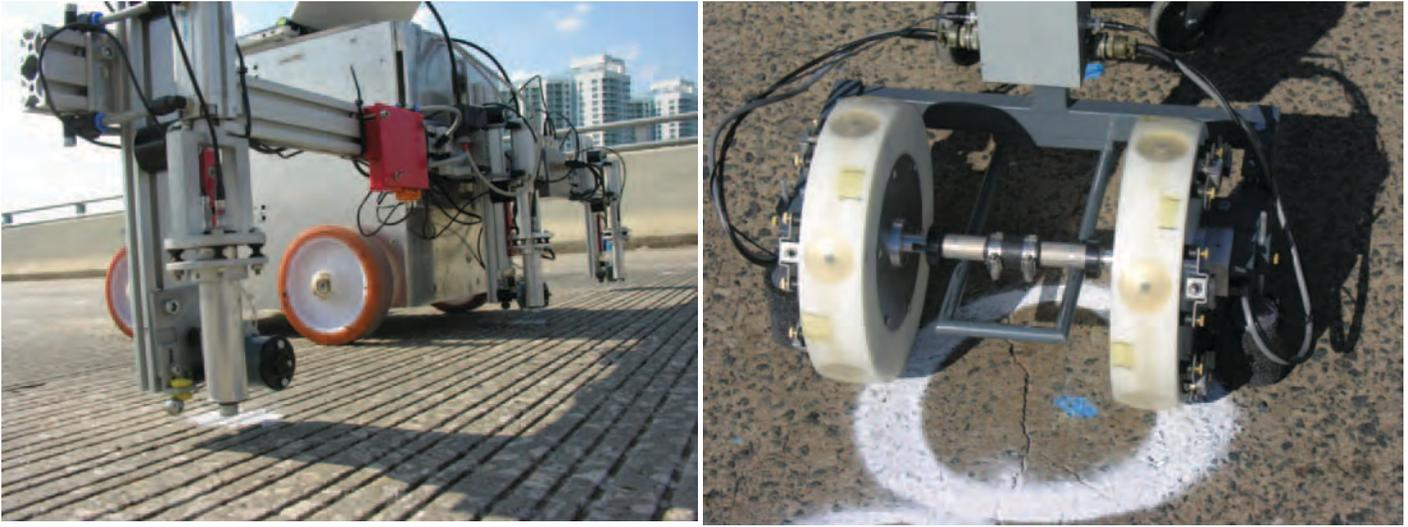
Figure 3.1. Stepper (left) and bridge deck scanner (right).
