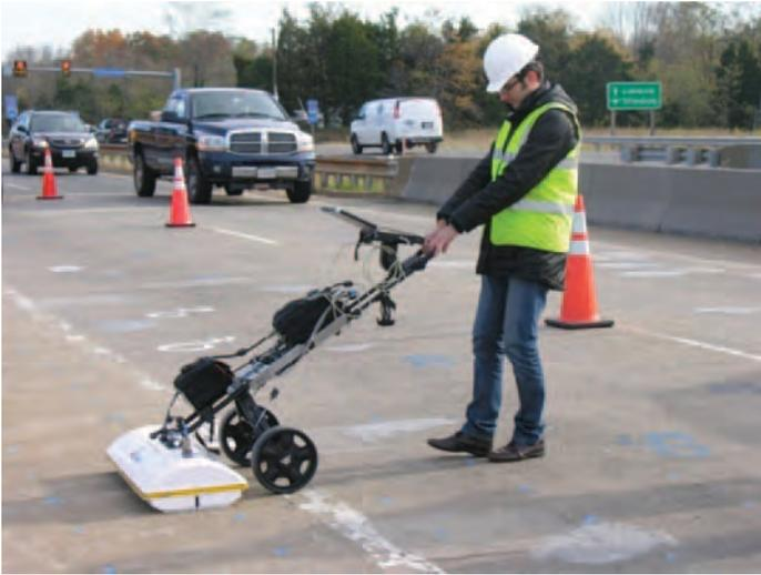
**Figure 5.7. Ground-penetrating radar: IDS.**
