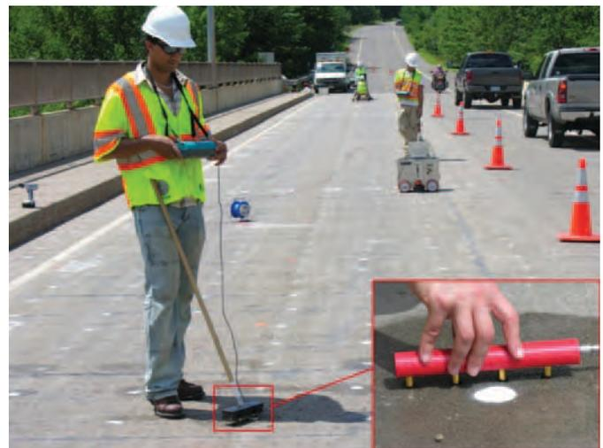
**Figure 3.16. Electrical resistivity testing using a Wenner probe.**
