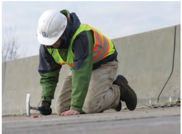
**Figure 3.21. Chain dragging (left) and hammer sounding (right).**
