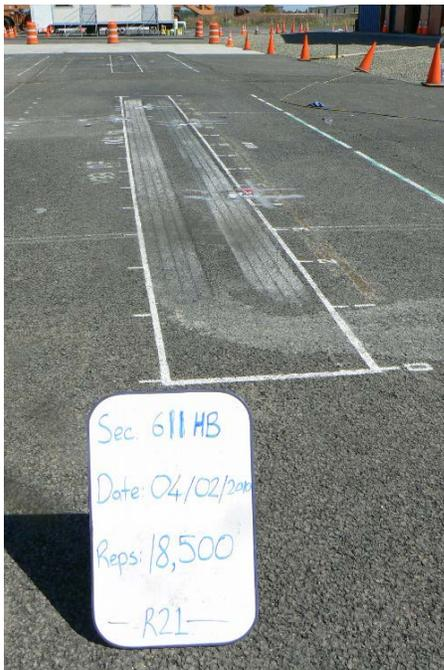
**Figure L.41. Photograph at test completion of Section 611HB, RHMA-G, 114 mm.**
