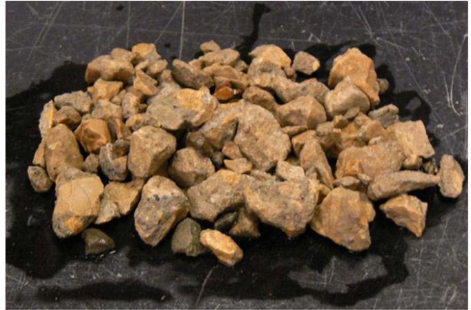
**Figure T.6. Limestone industrial crushed RCA wetted to distinguish natural aggregate from residual mortar.**
