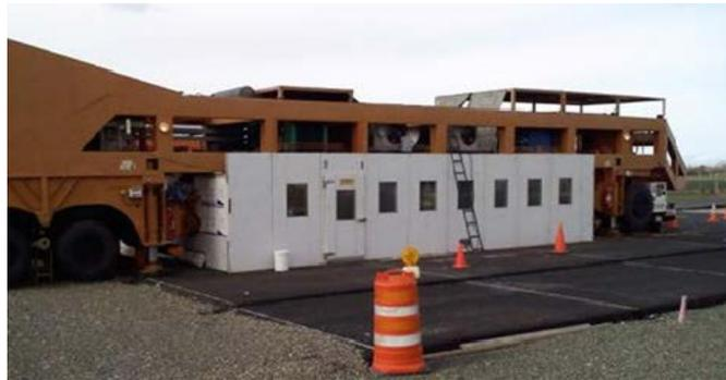
**Figure L.5. Specifications and photograph of HVS on SHRP 2 R21 test section at UCPRC.**
