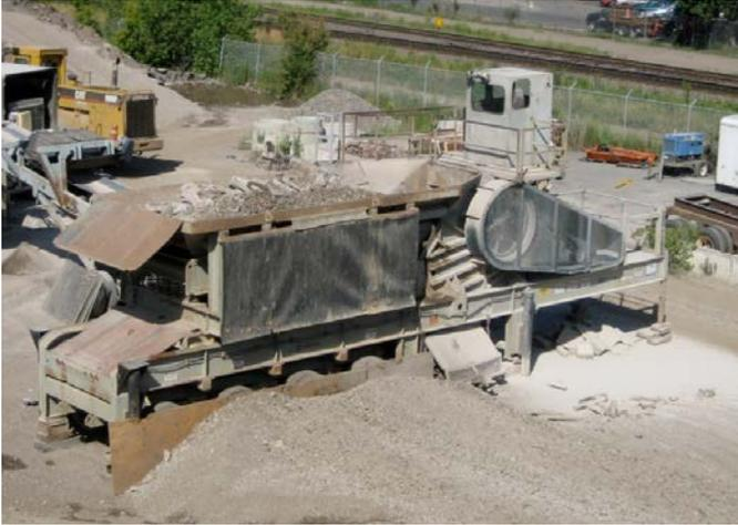
**Figure T.3. Jaw crusher used in the production of limestone industrial and I-94 industrial RCA.**
