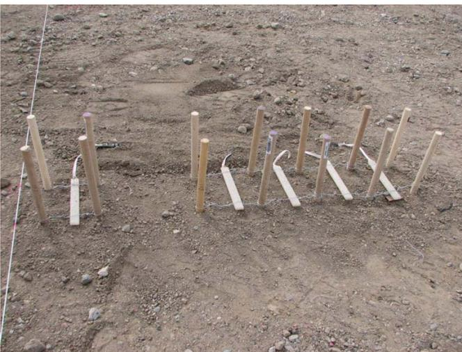
**Figure H.15. Dynamic strain gauge installation for Cells 71 and 72.**
