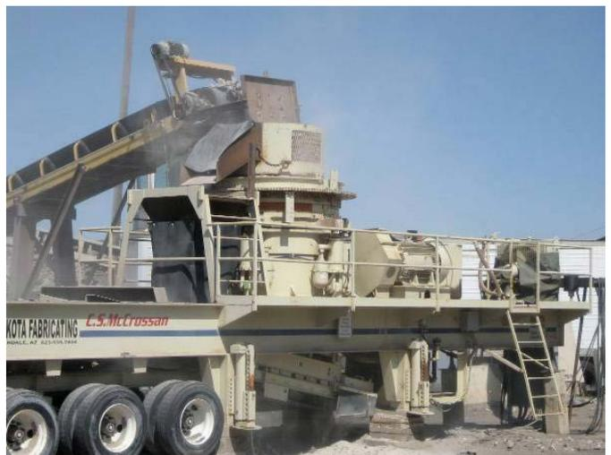
**Figure F.10. Cone crusher was used as secondary crusher to further remove the mortar from the natural aggregates.**
