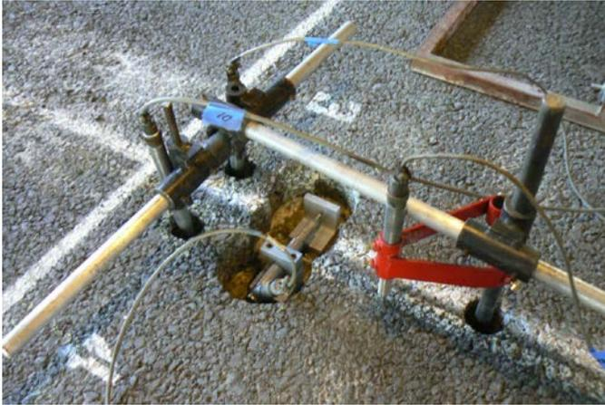
**Figure K.6.** Photograph shows JDMDs installed at traffic side (inner slab) near Joint J4. There are two vertical JDMDs on PCC, one horizontal JDMD on PCC, and one vertical JDMD on HMA.
