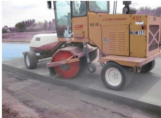
**Figure F.34. Treated surface and finishing platform (left); equipment for EAC brushing (right).**
