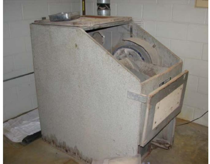
**Figure T.5. Jaw crusher used to produce I-94 laboratory-crushed RCA.**
