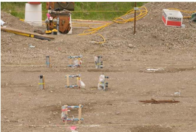
**Figure H.24.** An example of the sensors installed at midslab for Cells 71 and 72.
