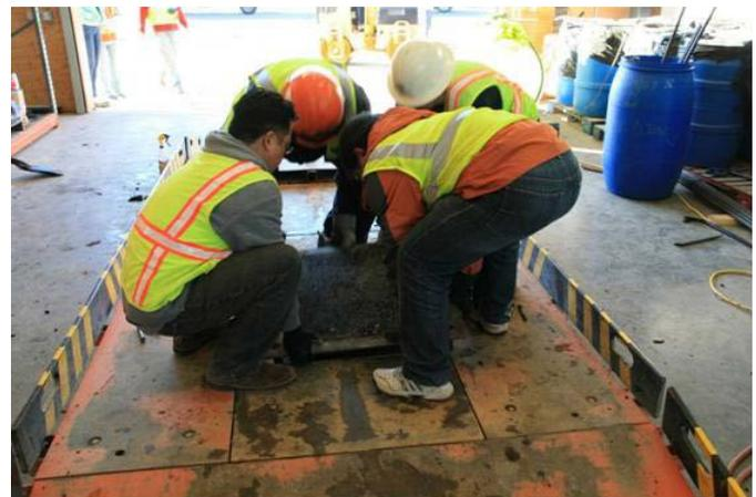
**Figure G.52. Removal of compacted HMA ingot, with a weight of approximately 150 lb.**
