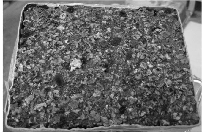
**Figure U.3. Scaled test surfaces of an EAC concrete sample after 56 freeze-thaw cycles.**
