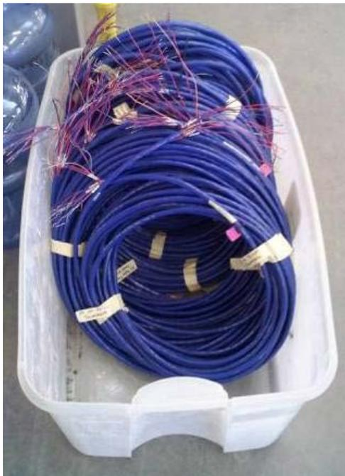
**Figure G.16. Thermocouple wire prepared for installation.**
