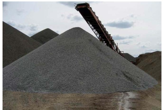
**Figure F.31. RCA stockpile being processed and saturated at a concrete recycling facility.**
