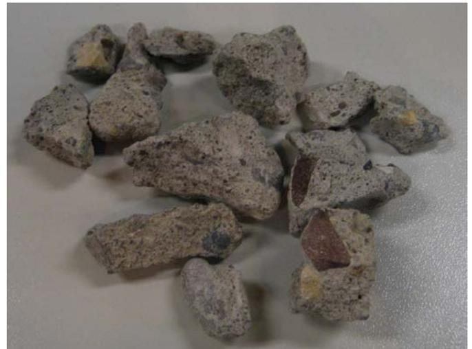
**Figure Q.3.** Laboratory-crushed RCA.
