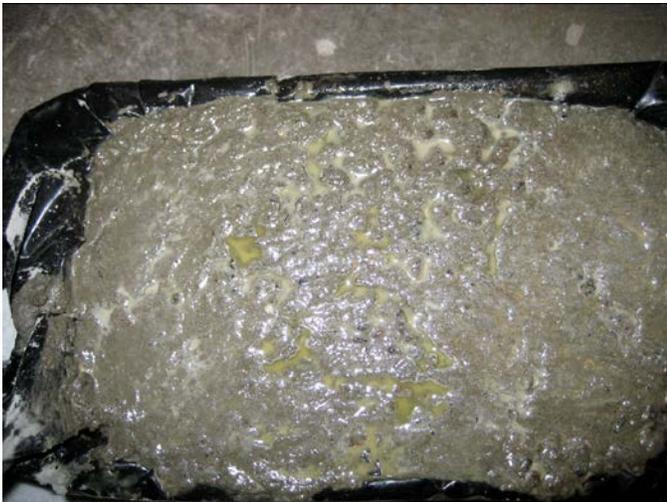
**Figure V.2. Specimen with Sika Rugasol-S surface treatment.**
