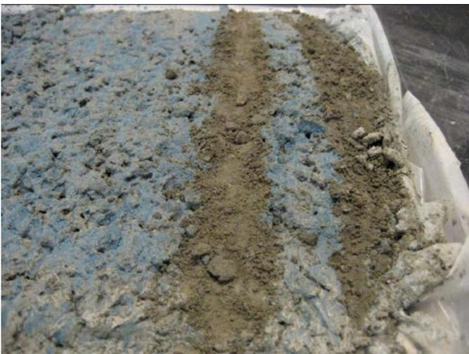
*Figure V.6. EAC-2 concrete specimen with curing/retarder BASF MBT Reveal. Scratches at 2 and 3 hours show that aggregate is easily removed from paste.*
