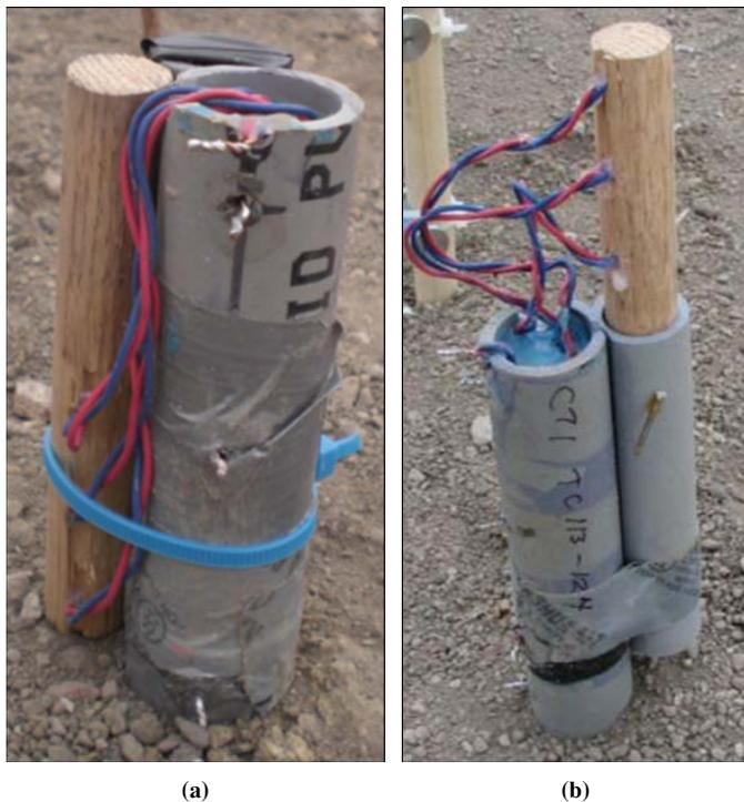
**Figure H.2. Thermocouple installed in Cells 71 and 72.**
