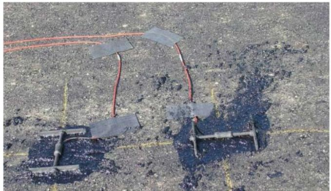
**Figure G.44. Sensors placed on bottom lift of PG 64-28PM, glued with mastic of sand and emulsion.**
