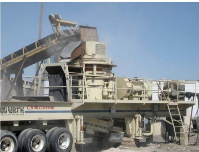
**Figure T.4. Cone crusher used in the production of limestone industrial and I-94 industrial RCA.**
