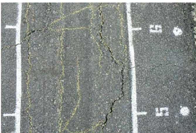
**Figure K.92. Section 614HB: Top view of the section between Stations 5 and 6 after completion of HVS testing. Transverse cracks (i.e., running left to right) can be seen. Chalk lines indicate hairline cracks visible at the pavement surface.**
