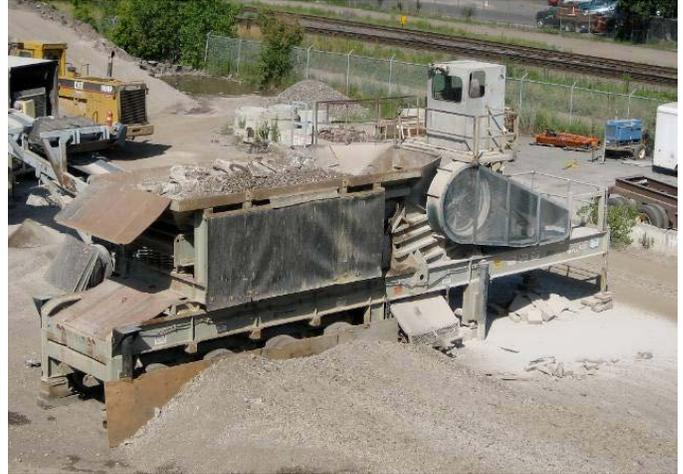
**Figure F.9. The primary crusher was the jaw crusher operating at less than full capacity.**
