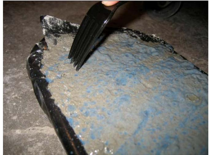
**Figure V.3. Brushing readiness test at 5 hours.**
