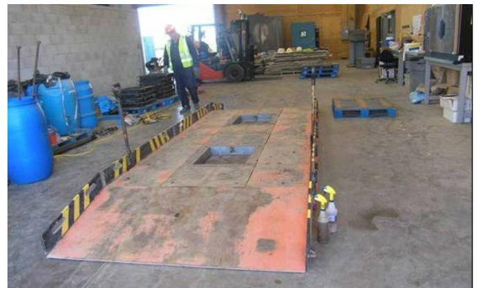
**Figure G.48. Assembled compaction frame and ingot molds for field mix-lab compact HMA specimens.**
