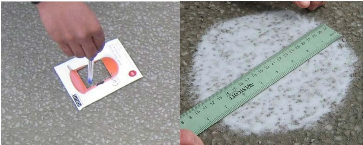
**Figure F.36. Quality control tests for brushing: (left) 25 cm<sup>2</sup> test to count aggregate peaks, and (right) sand patch test to determine texture depth.**
