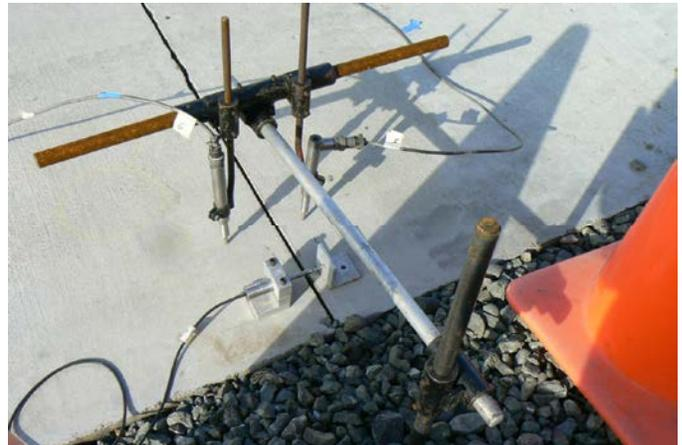
**Figure M.3. Photograph showing the JDMD configuration for monitoring both horizontal and vertical movements at a joint. The horizontal JDMD shown is model DSD800SE5 made by Daytronic, and the vertical JDMDs are model GHSD/GHSDR 750 made by Macro Sensors.**
