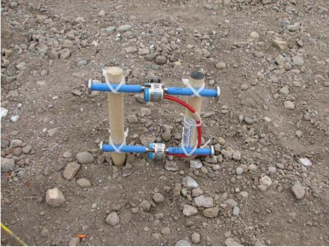
**Figure H.10. Static strain gauge installation for Cell 70.**
