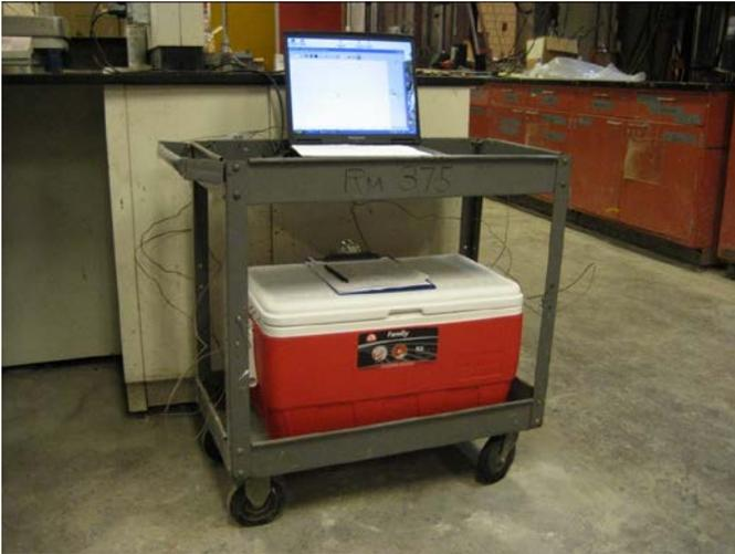
**Figure V.9.** Concrete temperature data acquisition system.
