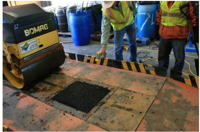
**Figure G.51. Compaction of ingots with rolling wheel compactor.**
