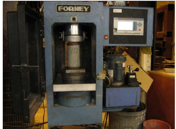
**Figure V.10.** EAC-3 cylinders were broken every hour from 5 to 10 hours, at 24 hours, and at 72 hours.
