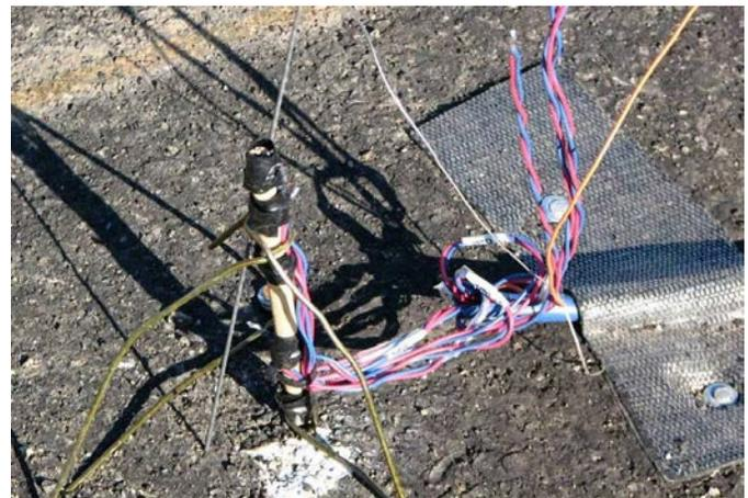
**Figure G.17. Close up of thermocouple placement on wooden dowel with wire mounting fixture before PCC placement.**
