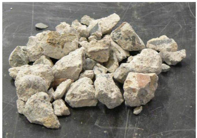
**Figure T.7. I-94 laboratory-crushed RCA.**
