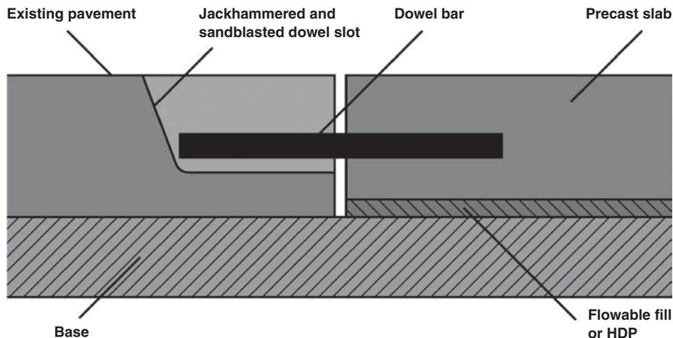
Note: Dowel bar caps should be used; HDP = high-density polyurethane.
