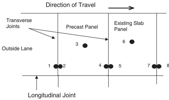
**Figure 3.1. FWD test locations for jointed systems.**
