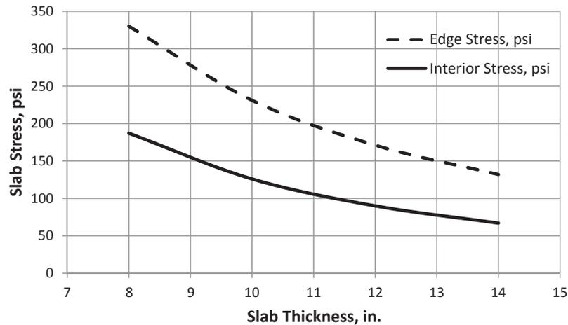
**Figure 8.4. Stresses as a function of panel thickness.**
