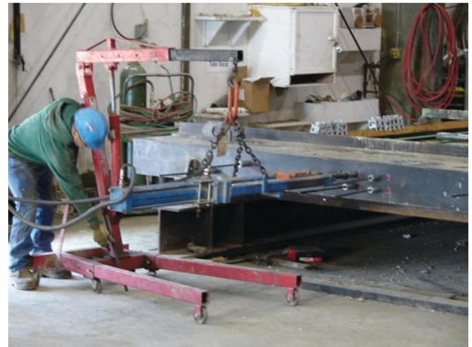
**Figure 9.8. Pretensioning process.**
