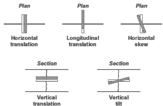
**Figure 5.3. Types of dowel bar misalignment.**
