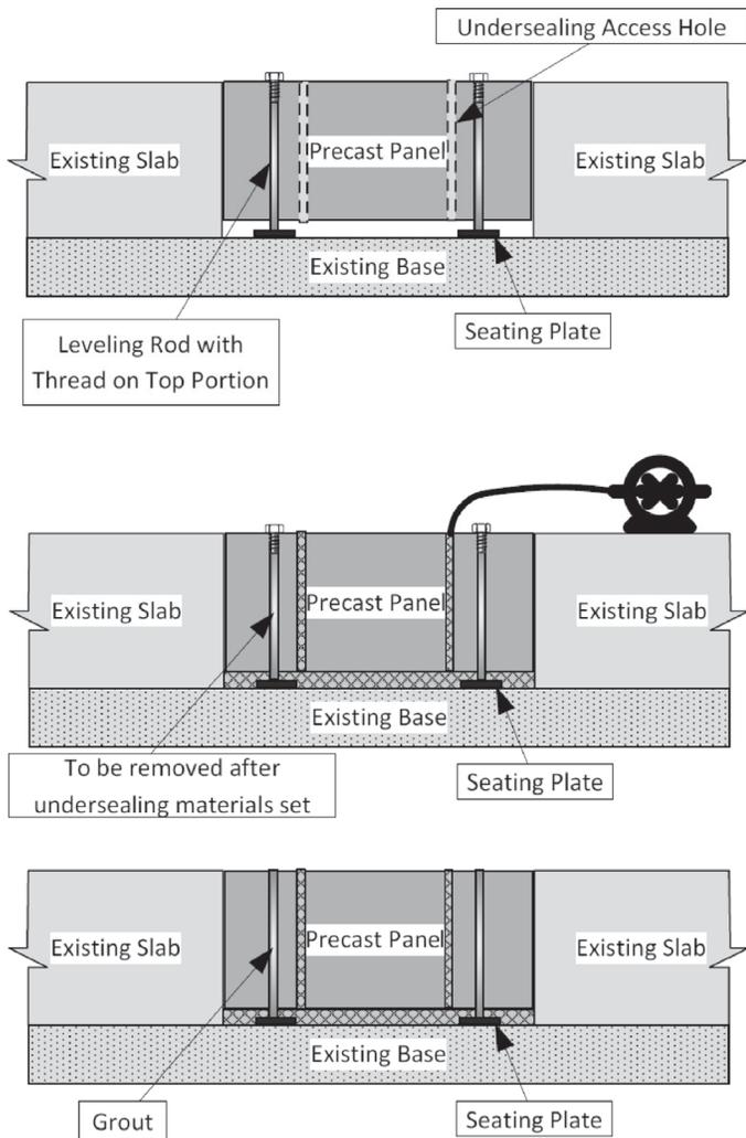
**Figure 10.5. Panel placement using threaded setting bolts.**
