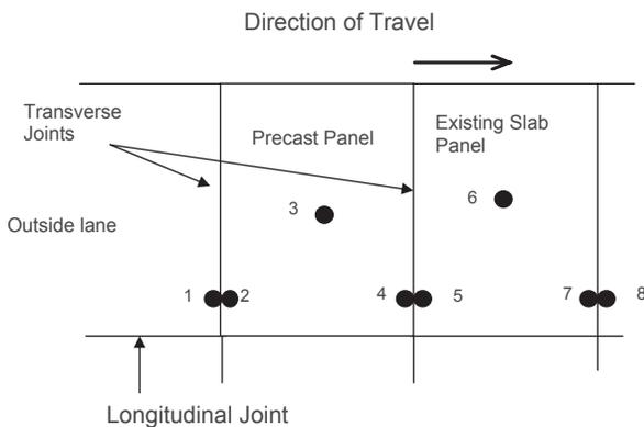
**Figure C.1. FWD test locations for jointed systems.**
