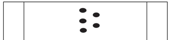
**Figure 12.6. Anchor locations in a longer central panel.**
