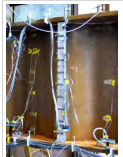
Figure 2: Deflection measurement device attached to web fold of corrugated girder
