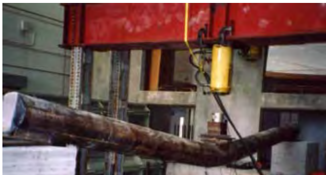
Figure 4: Concrete filled steel tube under loading
