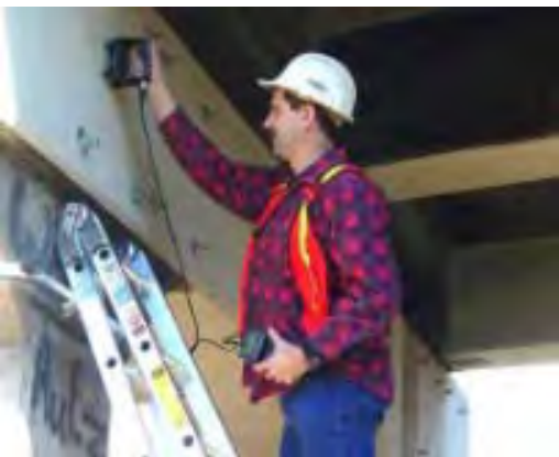
Figure 13: Impact echo measurements
