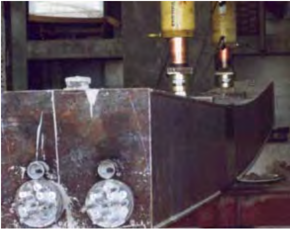
Figure 3: Bottom chord during loading
