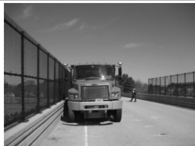
Figure 3: Load testing of bridge with design truck
