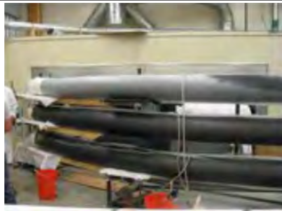
Photo 5. Tube bent around form during resin infusion
