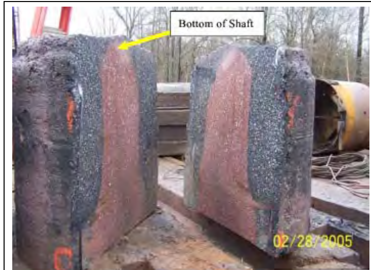
Figure 2: Longitudinal cut through bottom 6 foot section
