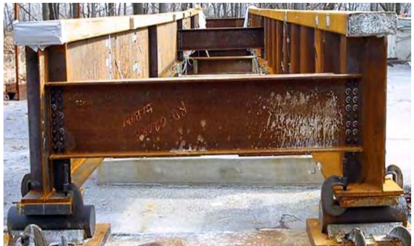
Figure 1: Concrete-filled tubular flange girder section
