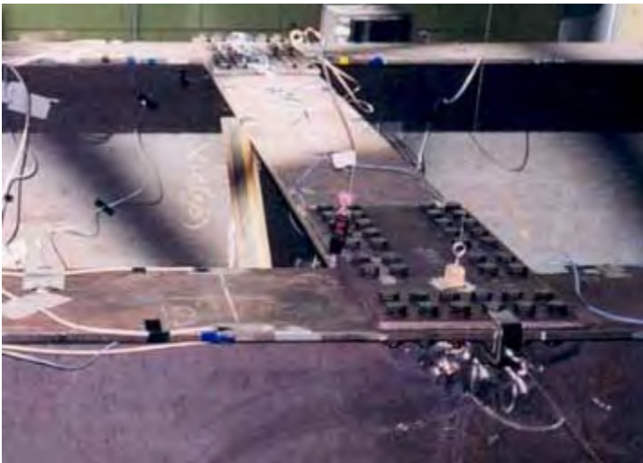
Figure 7: Set-up of flange rotational restraint testing
