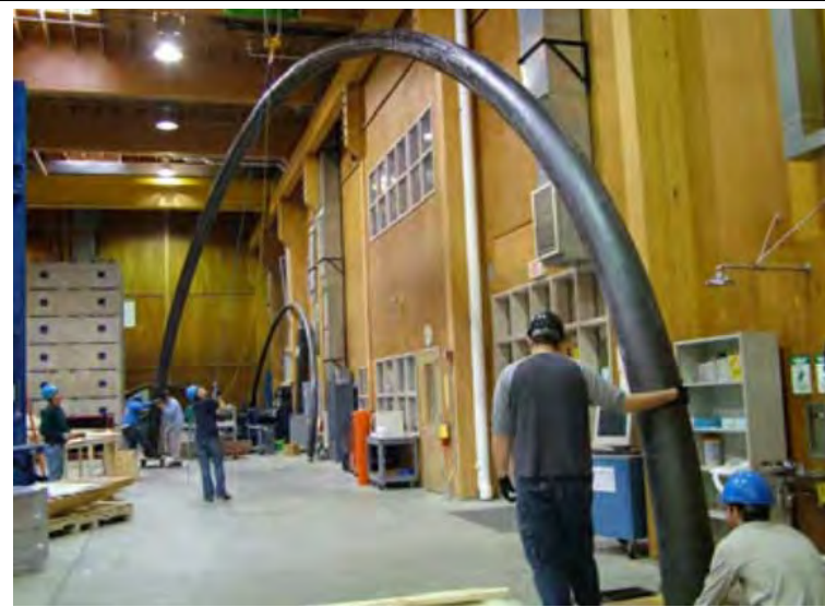
Photo 2: Finished FRP arch, light enough for two people to carry
