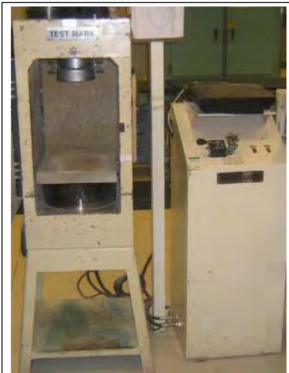
Figure 3: Load frame for testing compressive strength of concrete cylinders
