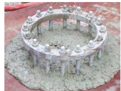
Figure 5: J-ring test patty
