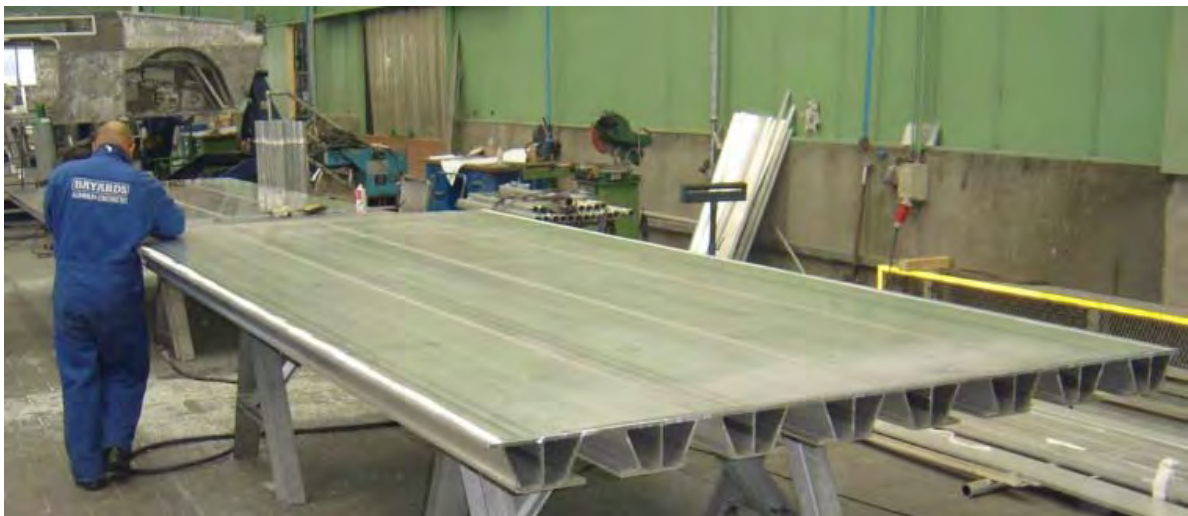
Figure 3: Fabrication of aluminum panels
