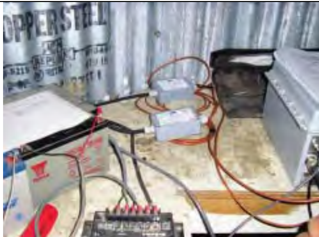
Figure 4: Transmission devices in streamgage shelter used to report channel-bed data
