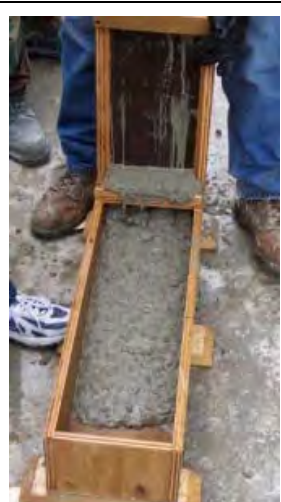
Figure 6: L-Box test after release of concrete
