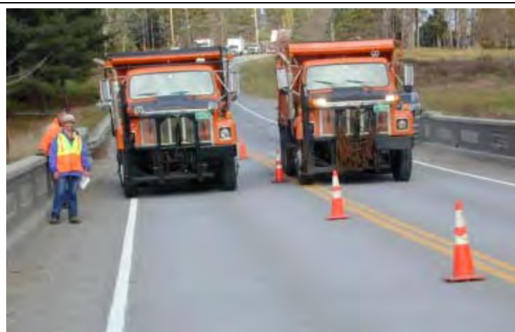
Figure 3: Load testing of bridge
