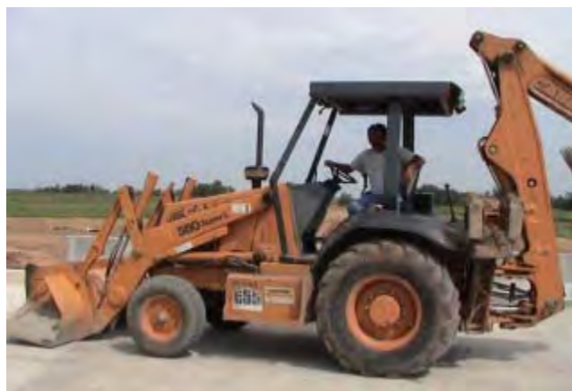
Figure 6: Backhoe used for serviceability acceleration testing
