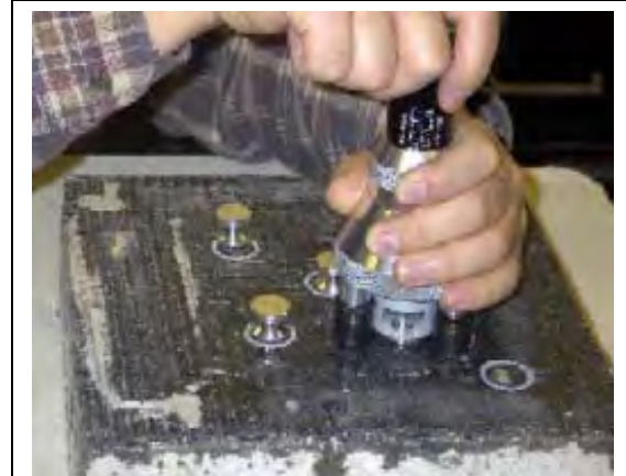
Figure 6: Pull-off test being performed
