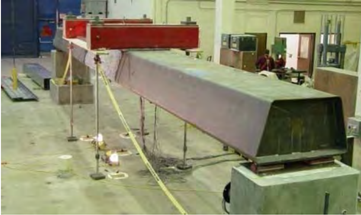
Figure 1: Folded plate girder during testing phase
