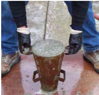
Figure 3: Inverted slump flow test
