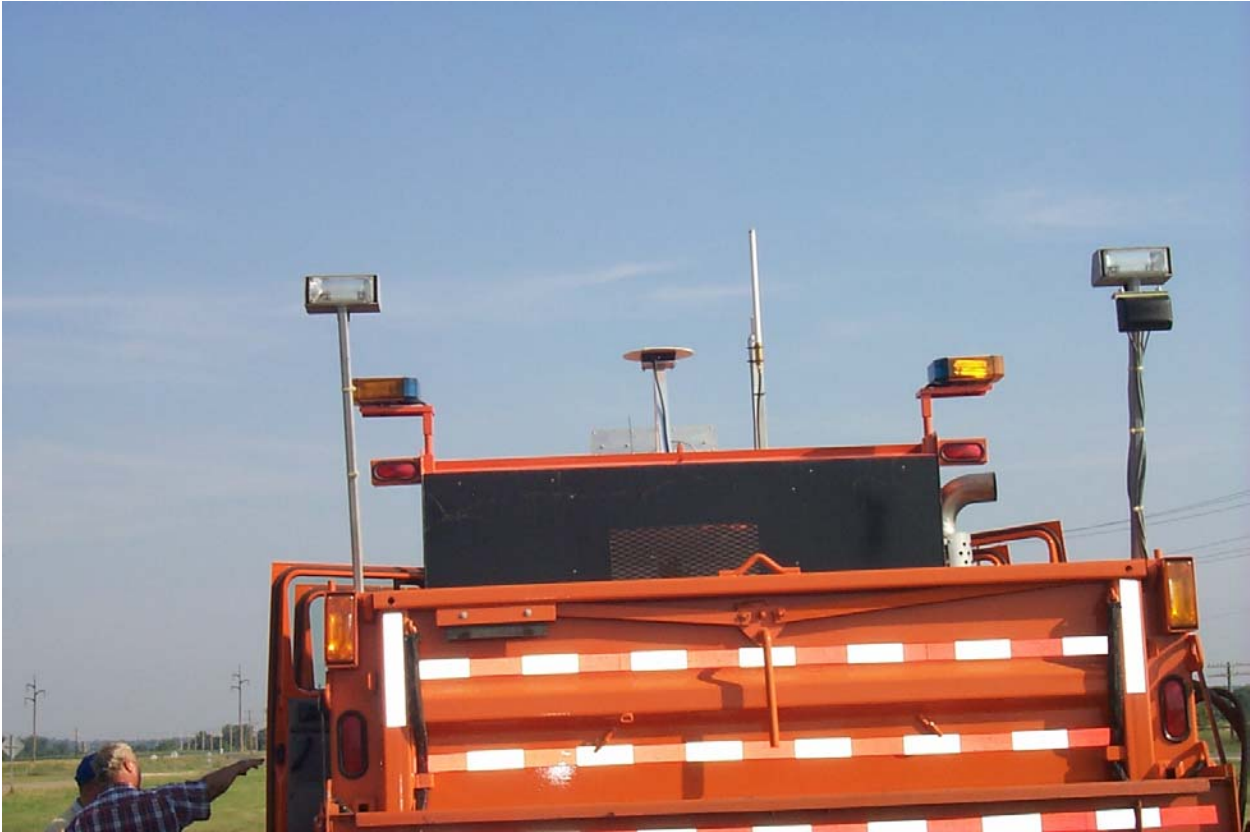
Rear radar/strobe collision warning system
