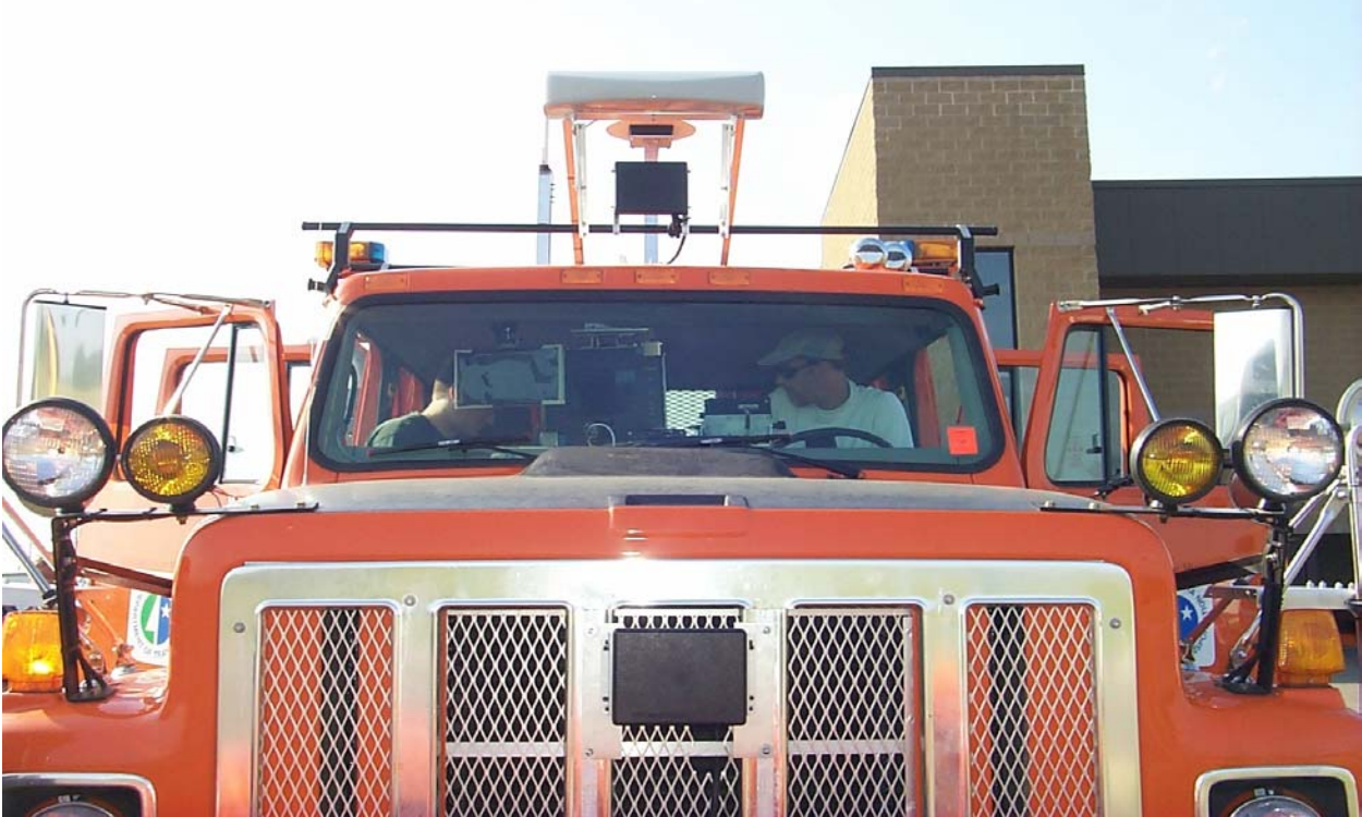
Front collision avoidance radar sensors (on grill and roof-mounted)
