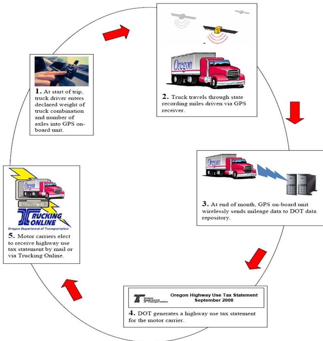
**FIGURE 2-4 Electronic weight-distance tax for heavy commercial vehicles.**
