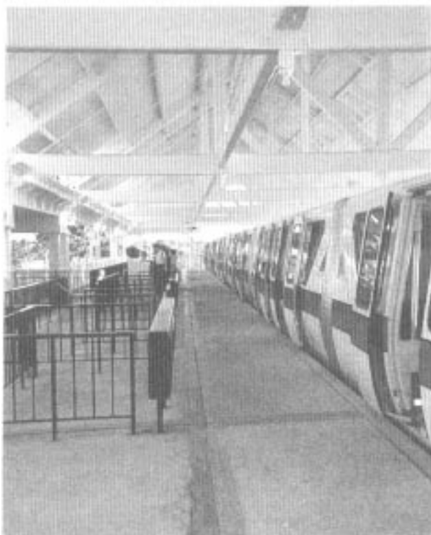
Figure 8. Platform gates and barriers on Disney World monorail system.
