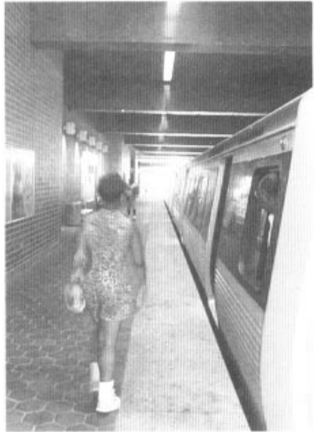
Figure 70. Passenger walking next to platform edge warning.
