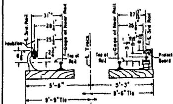
Location of Under-Running 3rd Rail, Bracket & Insulated Protection.
