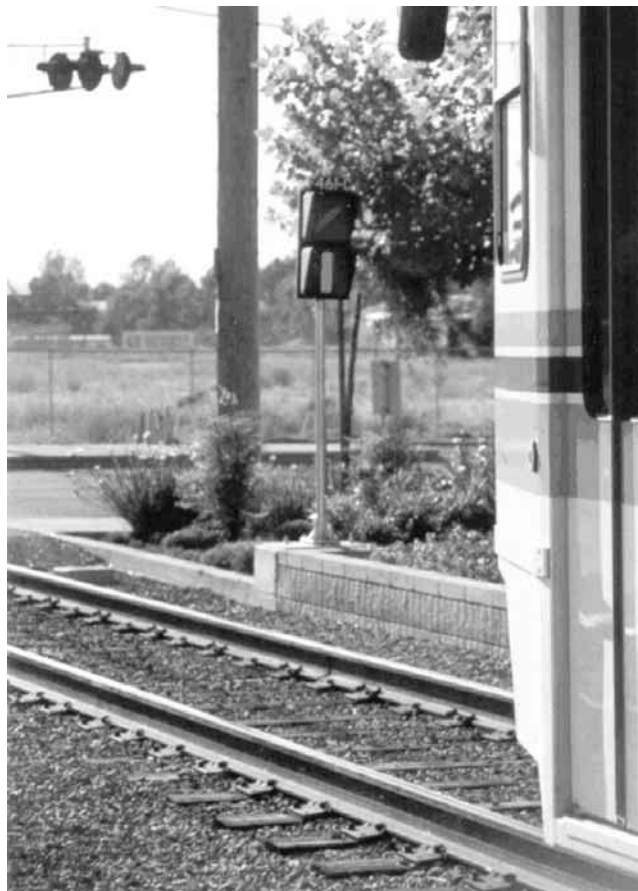
Figure 2-26. LRV operator gate indication signal. (Sacramento, California, 65th Street crossing.)
