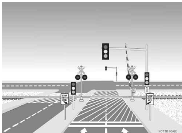
Figure 3-9. Presignal location at gated crossing.
