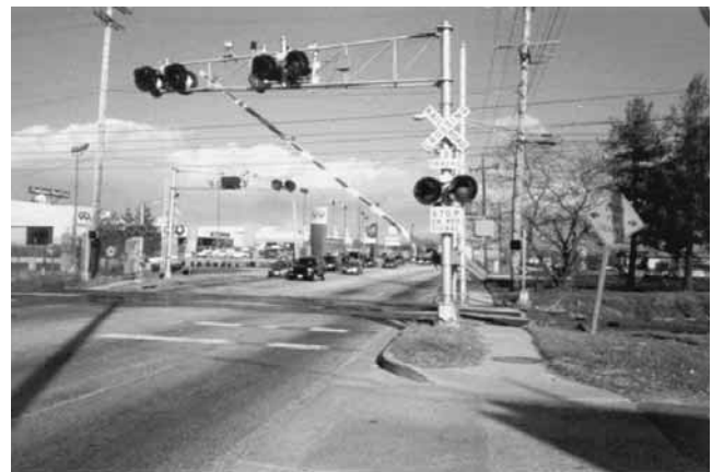
Figure 2-7. Second Train Approaching sign demonstration project site. (Baltimore, Maryland, Timonium Road crossing.)
