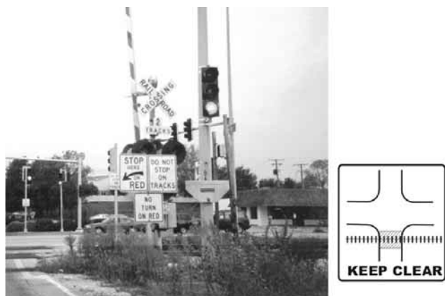
Figure 3-6. Example of sign clutter at an LRT crossing, with suggested design for alternative sign.
