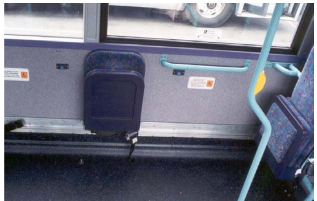
FIGURE 6 BC Transit rear-facing position with flip-down seats on bus wall and back panel.
