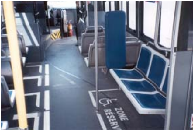
FIGURE 4 Montreal (Société de Transport de Montréal) rear-facing position adjacent to rear door, with stanchion to prevent tipping, designated priority markings on floor, and flip-up bench seating.
