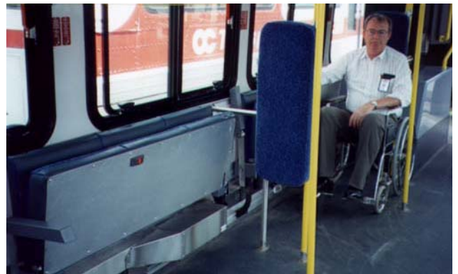
FIGURE 7 Ottawa (OC Transpo) rear-facing positions with stanchion and separate stop request button located under flip-up bench (in middle of bench underside).
