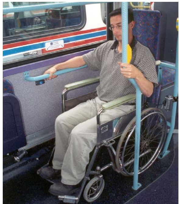
FIGURE 2 BC Transit rear-facing position with handrail and separate stop request button (located on wall below handrail).
