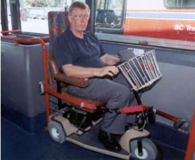
FIGURE 16 Two straps hooked together wrap around scooter in rear-facing position to prevent tipping, moving into the aisle, or rearward movement on BC Transit bus.
