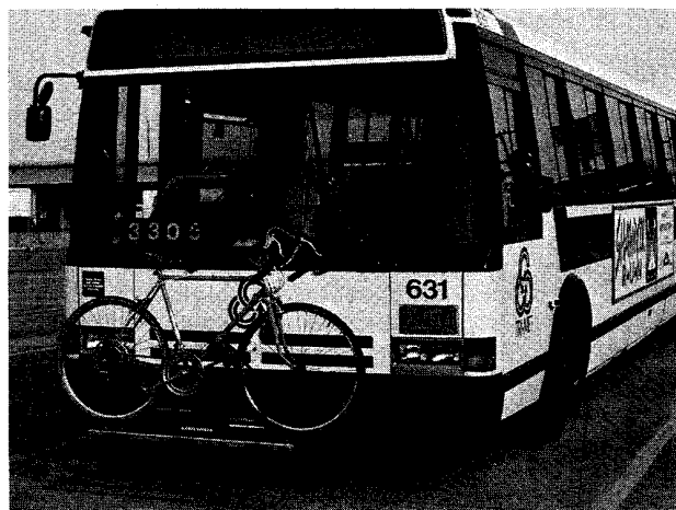
FIGURE 3 Mirror placement relative to bike rack (Courtesy of Tri-Met)
