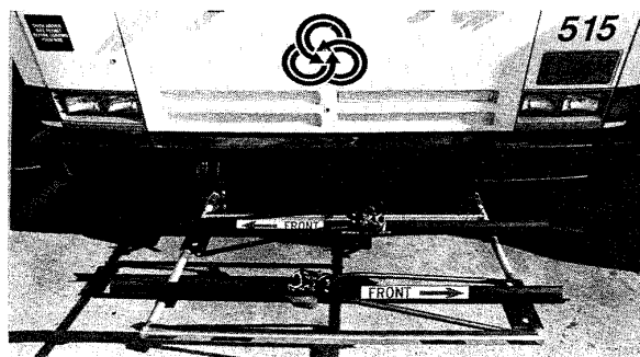
FIGURE 1 Example of a front-mounted rack for two bicycles. (Courtesy of Tri-Met)
