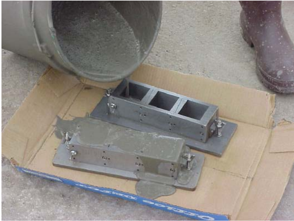
Figure 24 – 2” mortar cubes are made to test the grout strength
