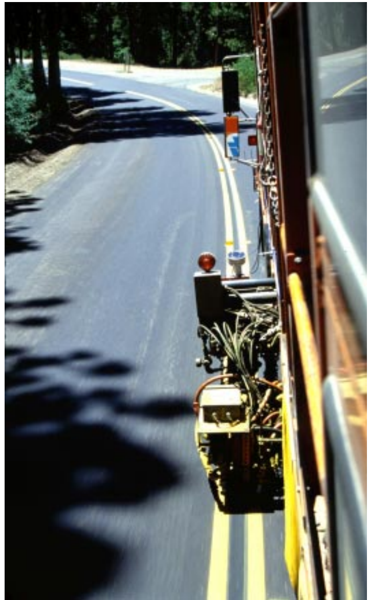
Figure 7. View from the rear operator's window showing the port outrigger in operation and shadows caused by trees adjacent to the roadway.
