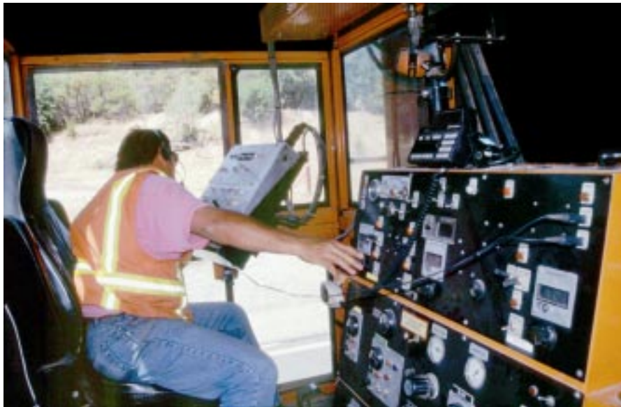
Figure 2. Caltrans lane restriping operator adjusting restriping controls while leaning out vehicle window to observe striping performance.
