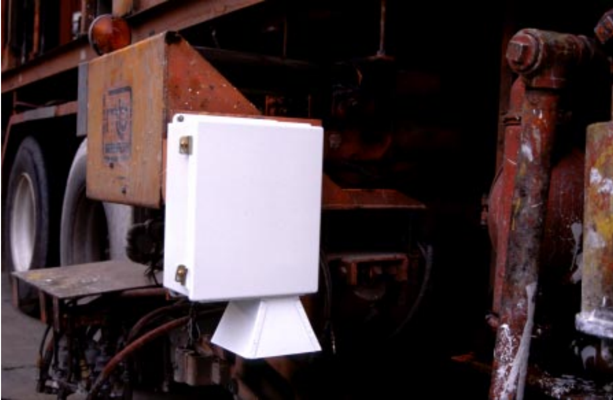
Figure 4. Machine vision system mounted inside the white enclosure attached to the edgeline outrigger on the starboard side of the striping vehicle with the outrigger in the normal operating position.
