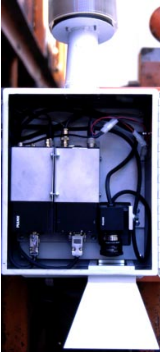
Figure 6. Enclosure interior showing the configuration of the two Zicam machine vision systems.
