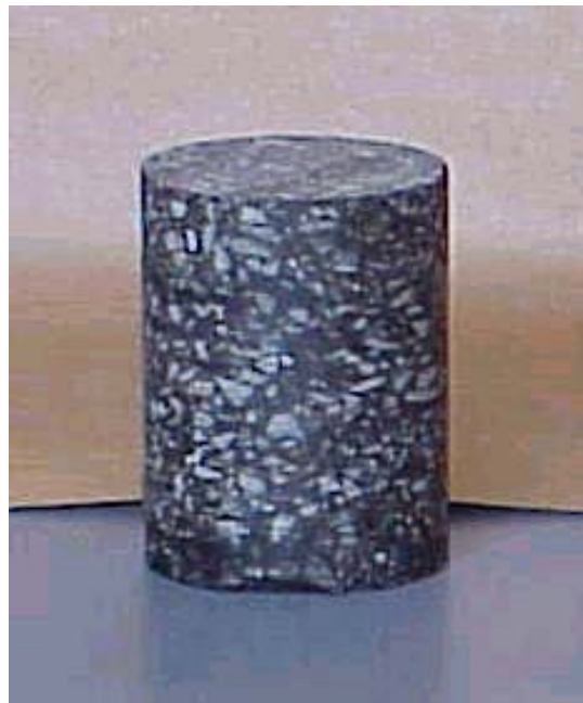
Completed Test Specimen 4 inch diameter, 6 inch height
