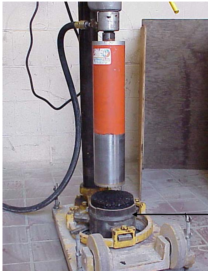
Photo 2 – Coring of Test Specimen
