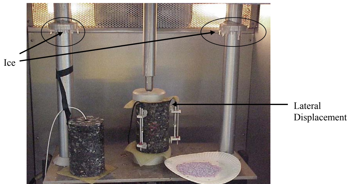
Photo 7 – Ice Formation on Testing Machine
