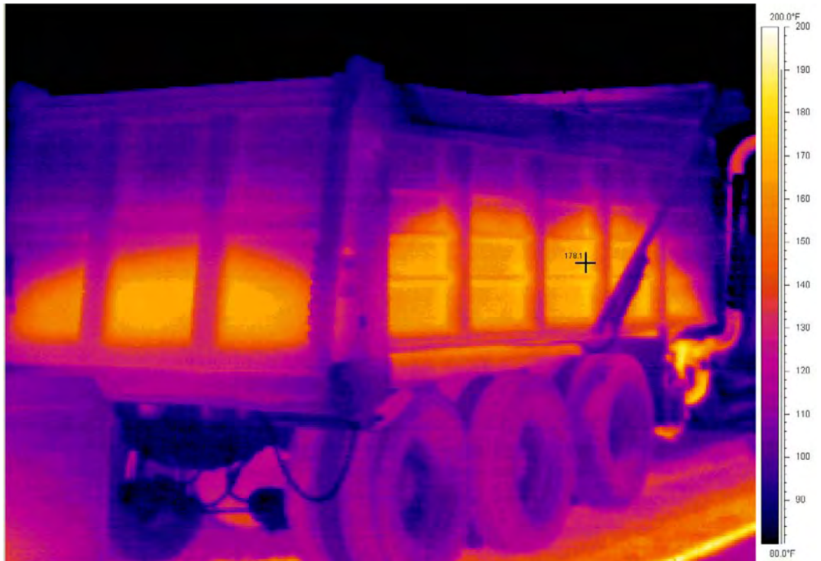
Figure A88 - Typical thermal image of a heated truck body
