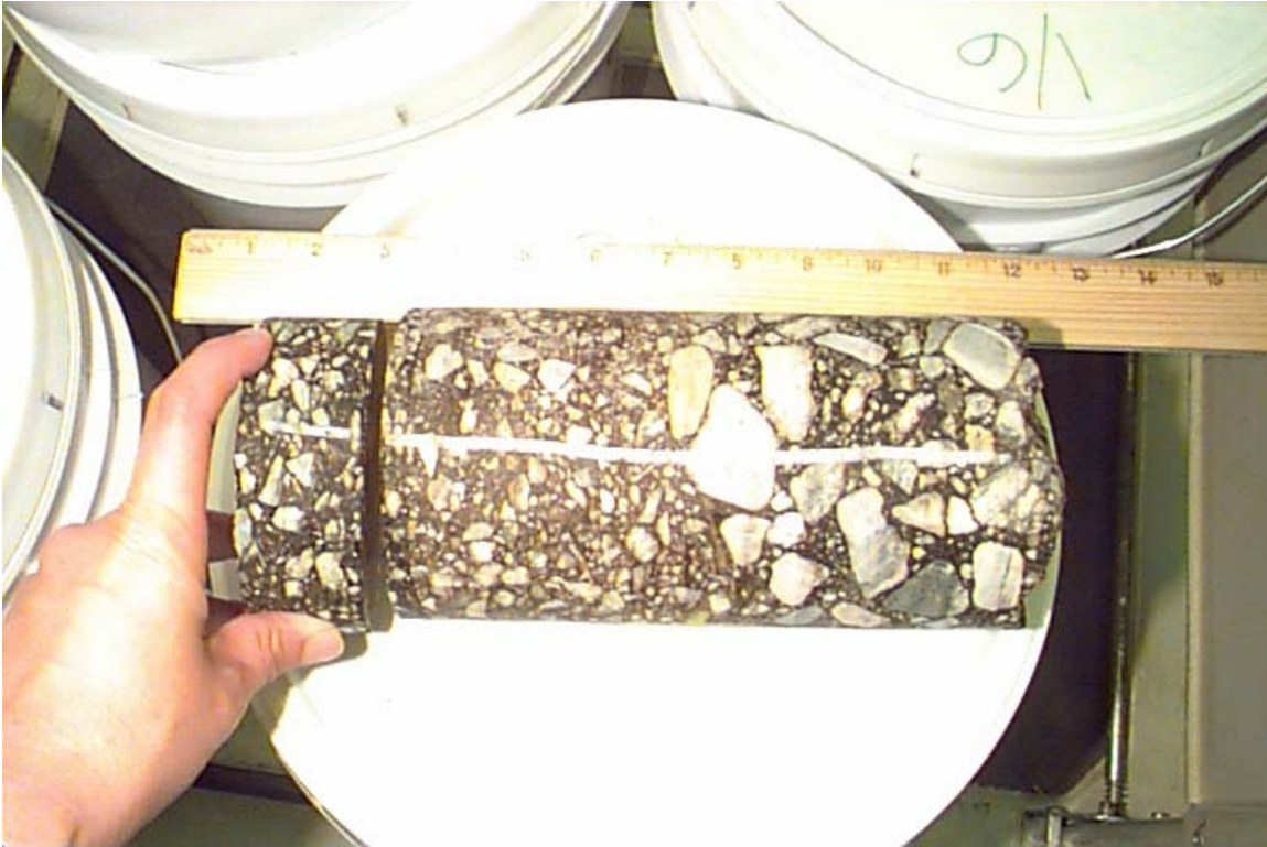
Image 12: Preparing Core Sample According to LTPP Protocols
