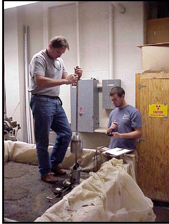
Figure 5.55 MaineDOT representative (operator #2) performing laboratory PFWD measurements.
