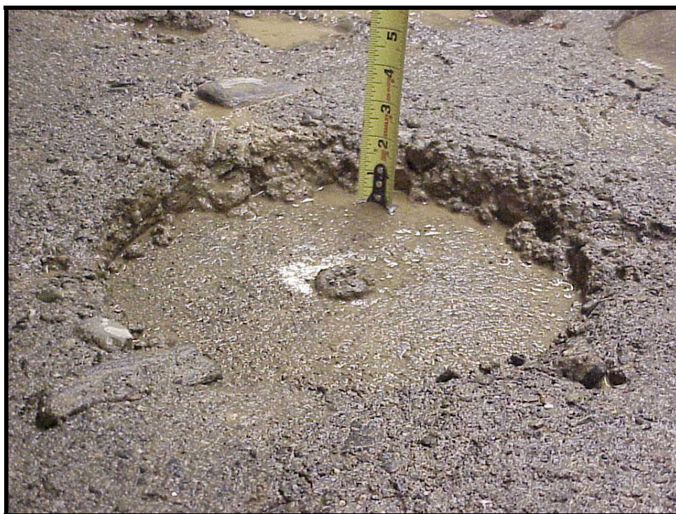
Figure 5.34 Prima 100 PFWD measurement on Wardwell gravel wet of optimum.
