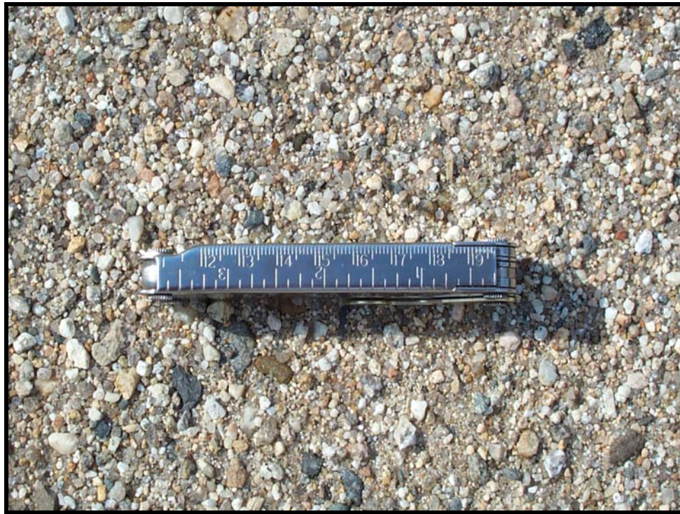
Figure 5.46 Poorly graded New Hampshire sand.
