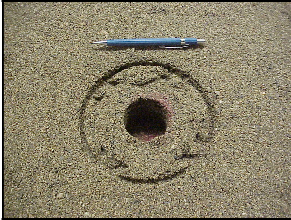
Figure 5.53 Clegg Impact Hammer measurement on New Hampshire sand.
