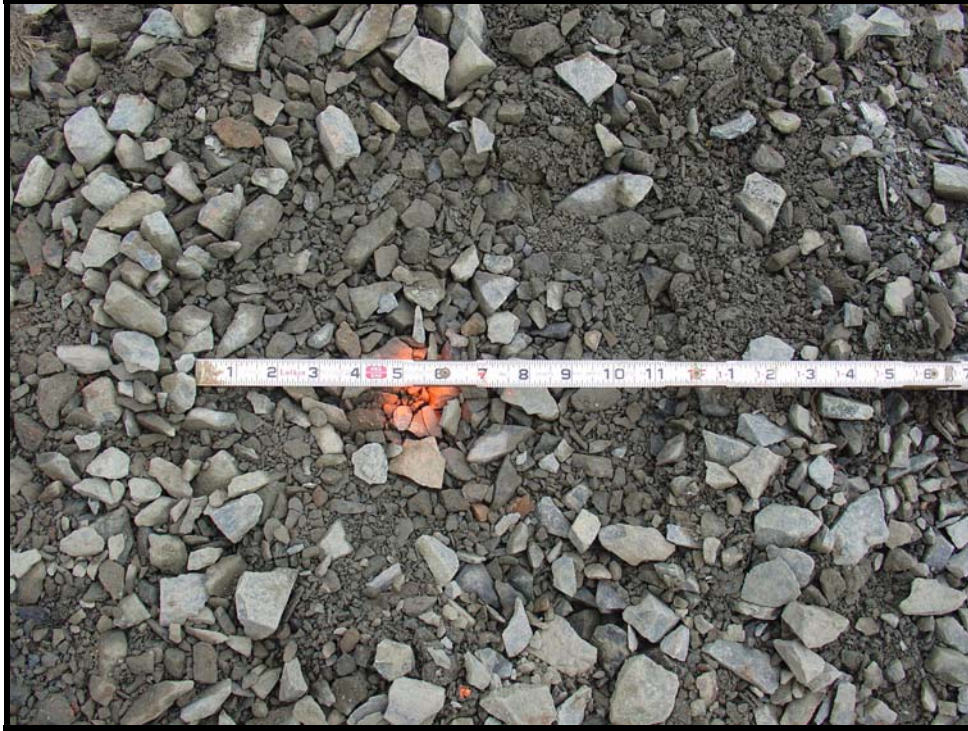
Figure 5.47 Well graded Connecticut crushed gravel.
