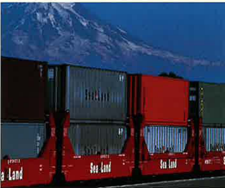
Railroad cars carrying double stacks of containers have made intermodal rail service more efficient and economical. Trainloads of containers cross the nation daily carrying products being shipped to foreign markets and imports for American consumers.
