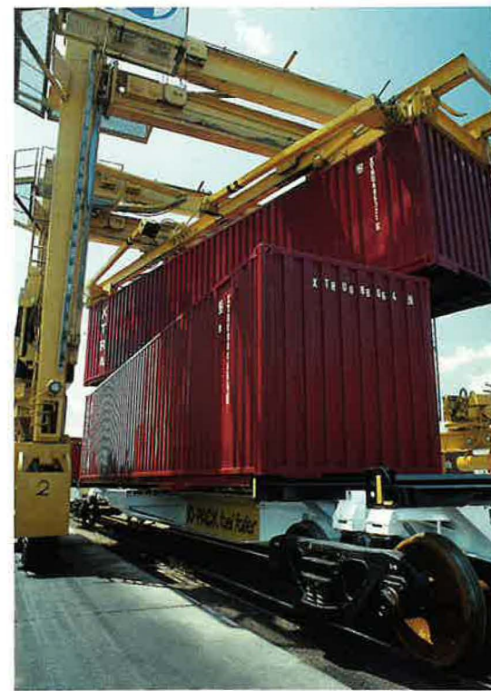
Straddle carriers position containers on railcars for inland distribution.
