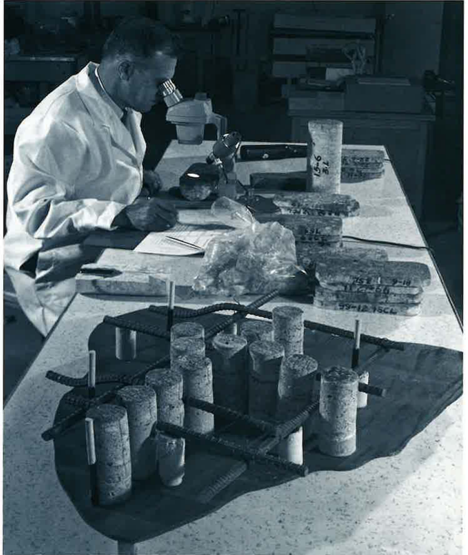
A geologist analyzes concrete pavement cores (circa 1950).
