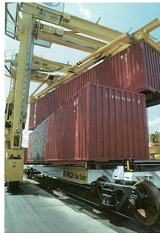
Straddle carriers position containers on railcars for inland distribution.
