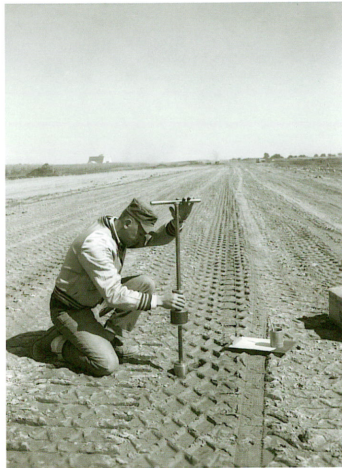
The AASHO Road Test, initiated in 1955, was managed by the Highway Research Board. Members of the HRB National Advisory Committee inspect the site in Ottawa, Illinois (top); a technician takes a field density sample (bottom).
