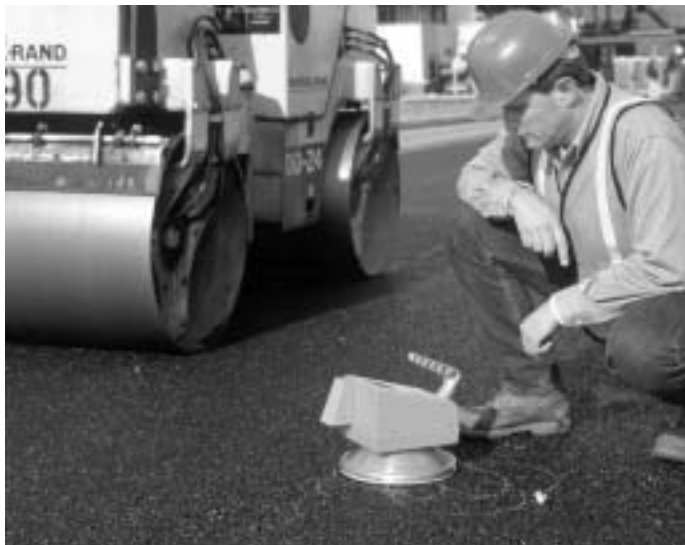
The 16-pound TransTech Systems Pavement Quality Indicator measuring density.
