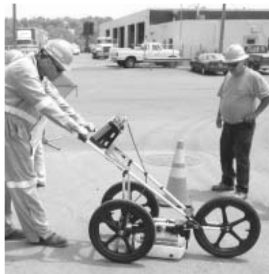
Ground-penetrating radar instrument locates and inspects utilities, part of maintenance quality assurance.
