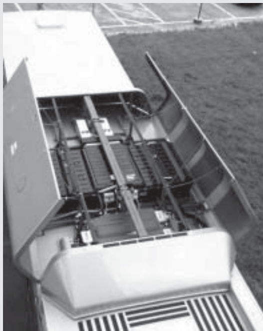
Electric storage system of a hybrid gas-electric bus, now being tested by CTTransit in Hartford, Connecticut.
