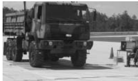
Demonstration of weigh-in-motion (WIM) at Fort Bragg, North Carolina, May 2003, with truck moving over portable system.
