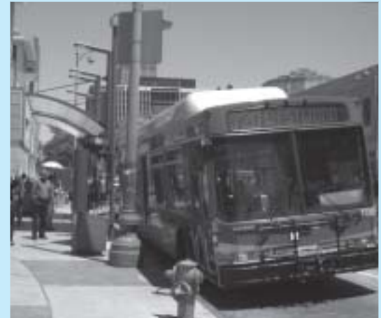
The Metro Rapid BRT, operated by the Los Angeles County Metropolitan Transit Authority, speeds up commuter time by making fewer stops and running more frequently; special transponders cause traffic signals to favor the bus, and low-floor designs allow faster boarding and alighting.
