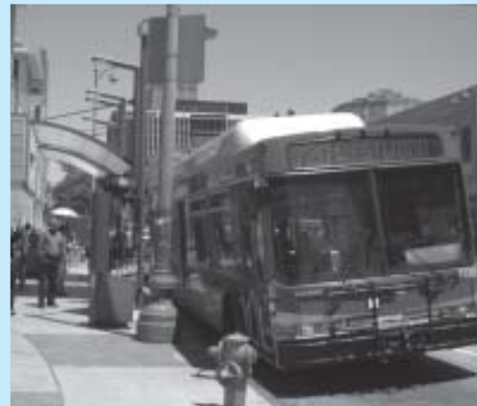
The Metro Rapid BRT, operated by the Los Angeles County Metropolitan Transit Authority, speeds up commuter time by making fewer stops and running more frequently; special transponders cause traffic signals to favor the bus, and low-floor designs allow faster boarding and alighting.
