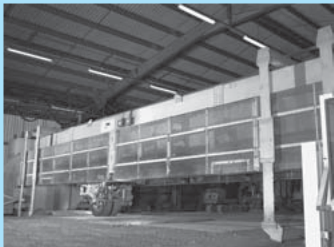
Pavement test facility at Transport Research Laboratory, United Kingdom, is used to test and evaluate the durability of materials under roadway loading conditions. COST has developed a code of good practice for testing facilities to improve the application of results.
